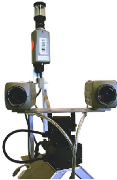
Figure 8.6.: Vision system of TASER consisting of Sony DFW-VL 500 mounted on the pan-tilt-unit PTU-46-17.5 and an omnidirectional camera. Source: (Jockel, 2009).
