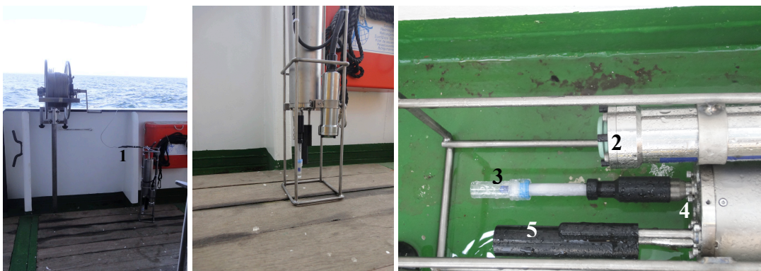
Image C06: Winch and CTD probe (left) and sensing elements (middle and right). Number through images: 1) data transfer and power supply cable and connection an rope of winch; 2) Oxygen sensor; 3) temperature probe; 4) pressure sensor; 5) conductivity cell.
