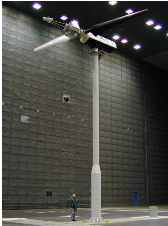
Figure 3.7.: The wind turbine model in the Ames wind tunnel. From http://wind.nrel.gov/amestest/Wconfig.htm
