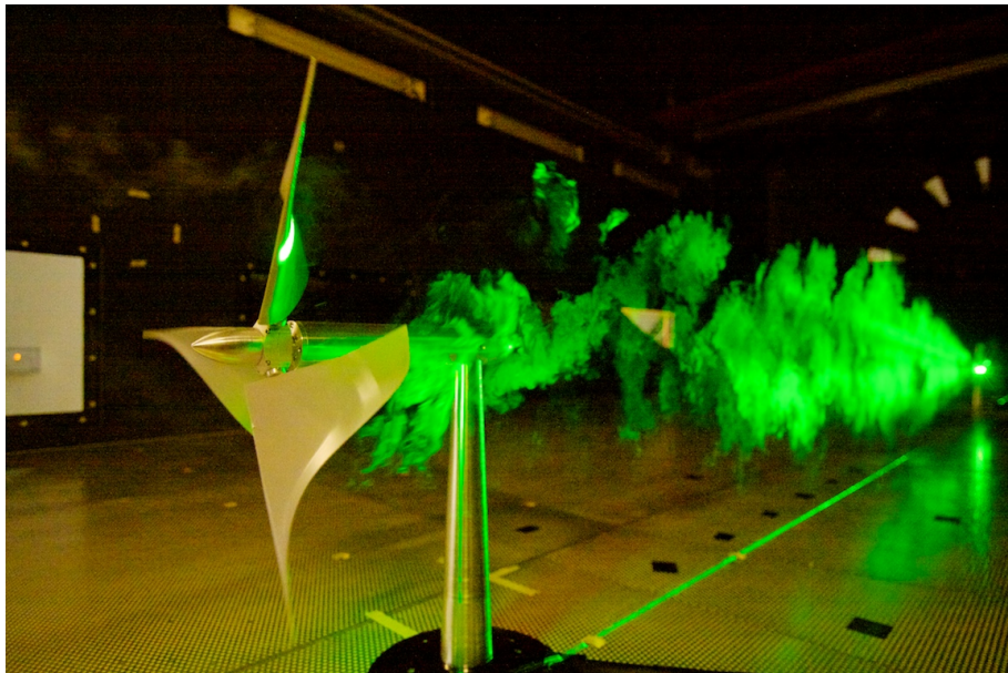
Figure 8.6.: Wake flow visualization - helical structures and far wake
