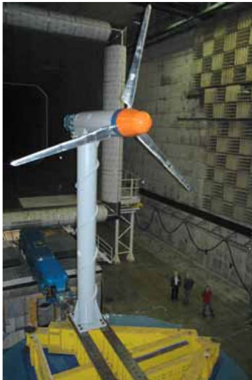
Figure 3.8.: Wind turbine model in the DNW wind tunnel, from Snel and Schepers (2007)
