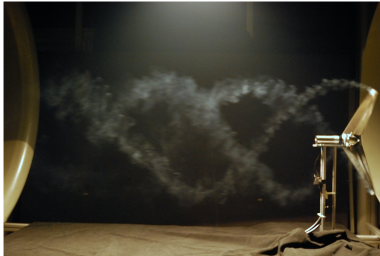
Figure 5.3.: Streaklines show the boundaries of the wake
