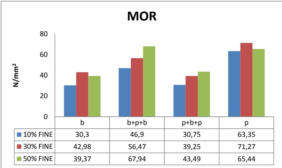
Figure 46. Average MOR of fines core layers of 16 mm OSB
