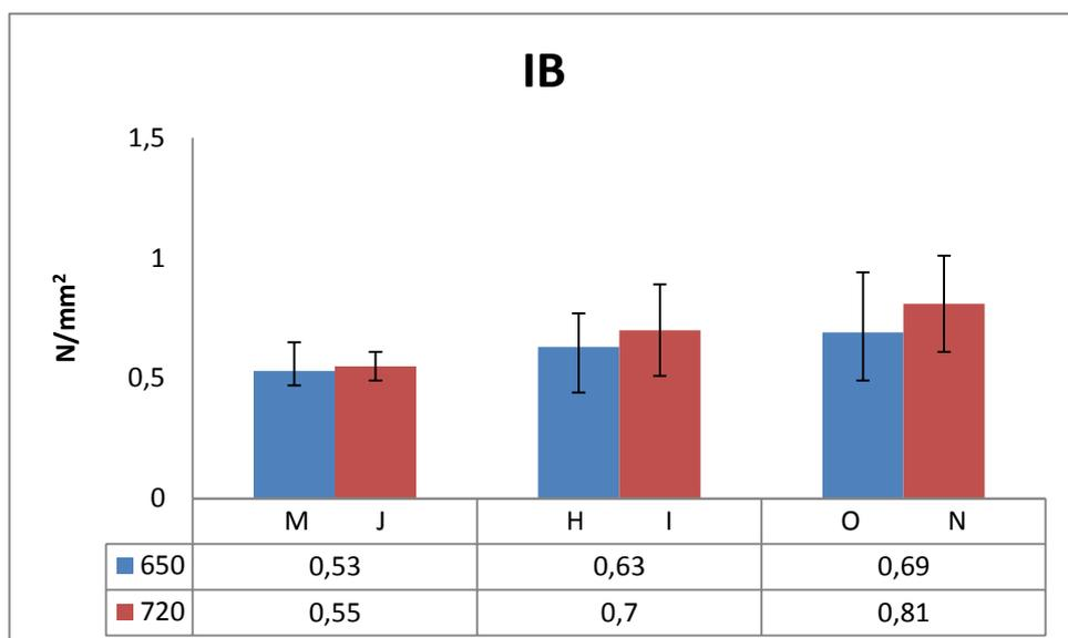
Figure 41. Average IB of beech strands based core 16 mm OSB
