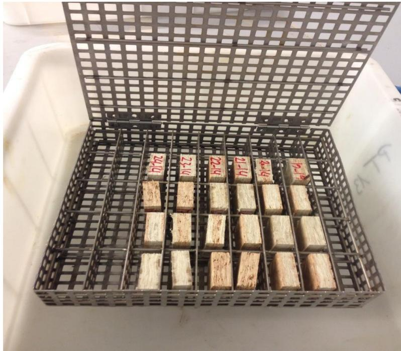
Figure 27. Steel frame for TS and WA measurement
