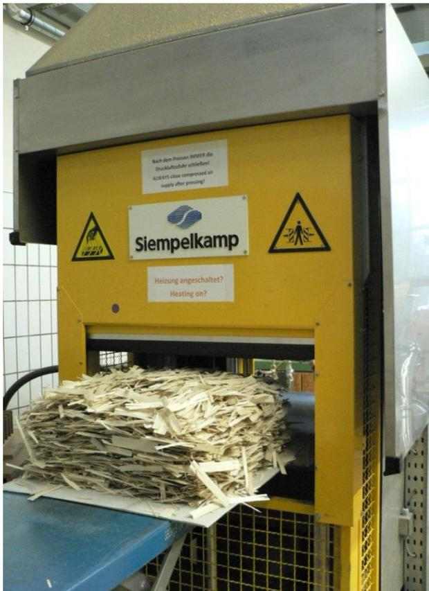
Figure 21. Feeding the hot press (without top press sheet)
