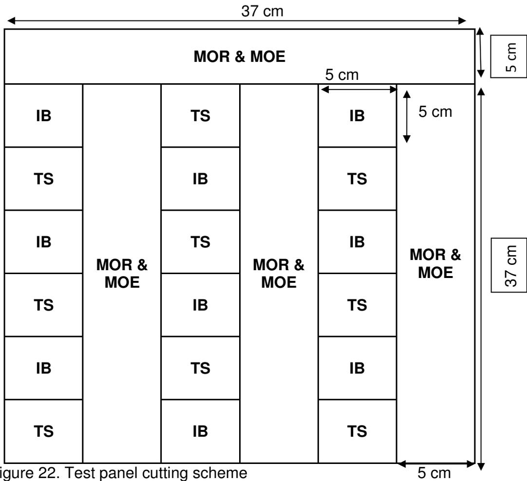
Figure 22. Test panel cutting scheme
