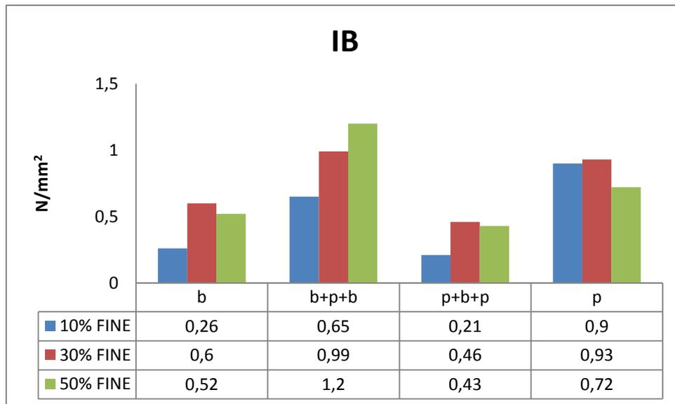
Figure 48. Average internal bond of fines core layer of 16 mm OSB
