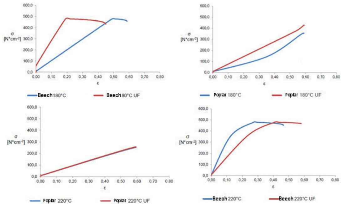
Figure 1. Stress Strain Diagrams of the Densification Experiments
