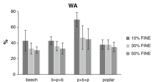
**Fig. 7** Average water absorption of fine core layers of 16 mm OSB. *b* beech, *p* poplar
