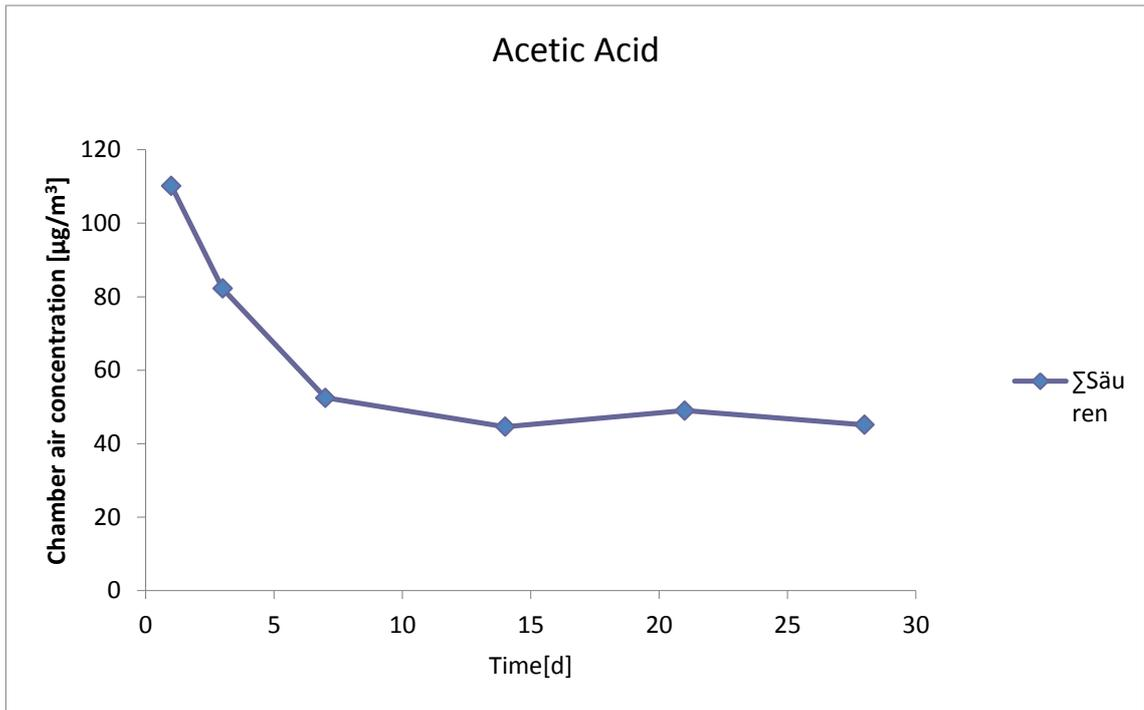
Figure 59. Acetic acid emission rate of solid poplar during 28 days of testing
