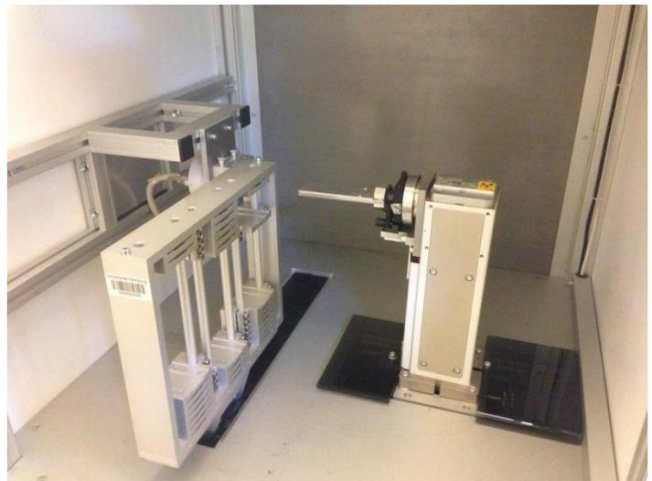
Figure 26. X-ray device for vertical density profile
