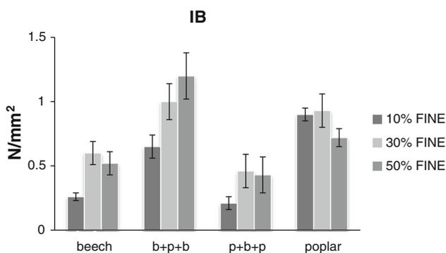
**Fig. 5** Average IB of fine core layer of 16 mm OSB. *b* beech, *p* poplar
