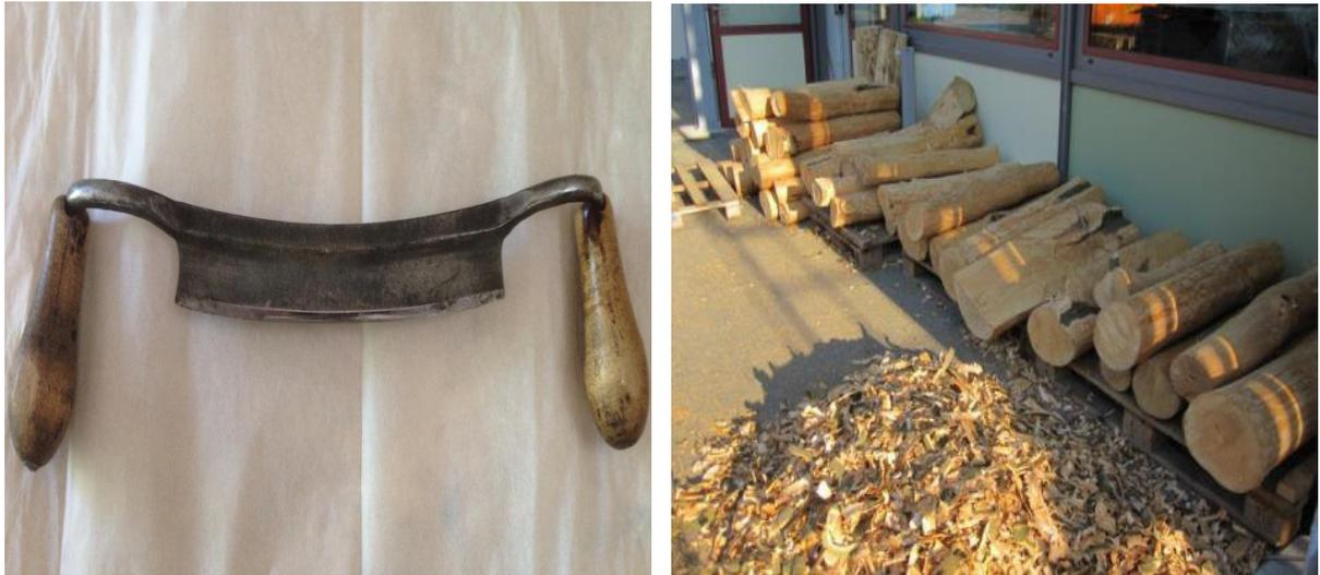
Figure 14. Knife device for debarking logs (left) and debarked logs (right)
