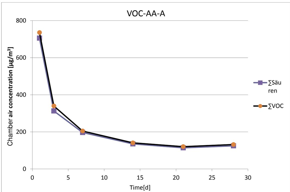
Figure 56. Total emission rate of solid beech during 28 days of testing
