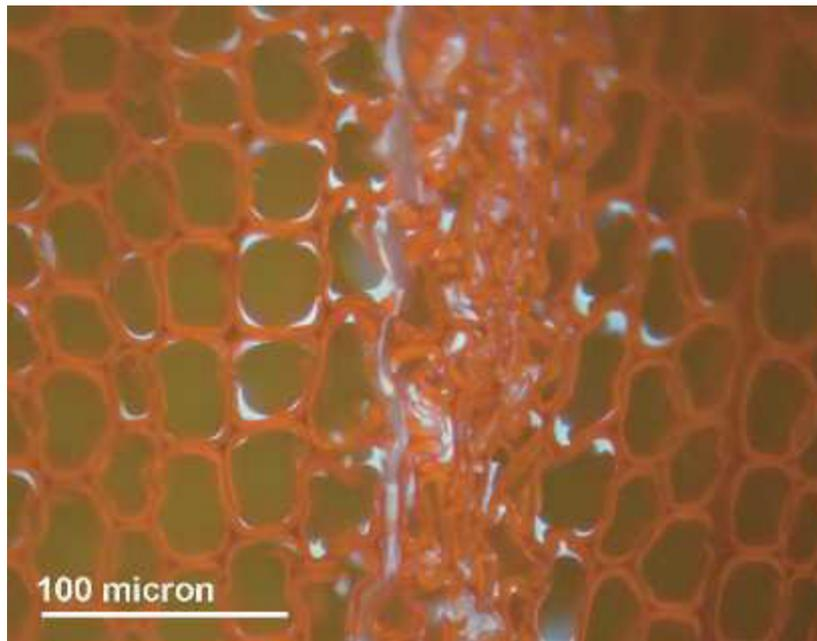
Figure 11. Photomicrograph of a MDI bondline in southern pine using epifluorescence and stained with 0.5% safranin O. Transverse view of vertical bondline. Bright areas are resin. Filter set 360-nm / 400-nm / 420-nm (Kamke 2004)
