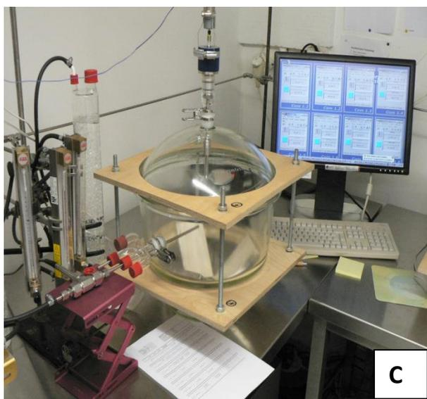
Figure 28. Sample preparation for VOC (A: Solid wood sample, B: OSB Sample) and C: Desiccator
