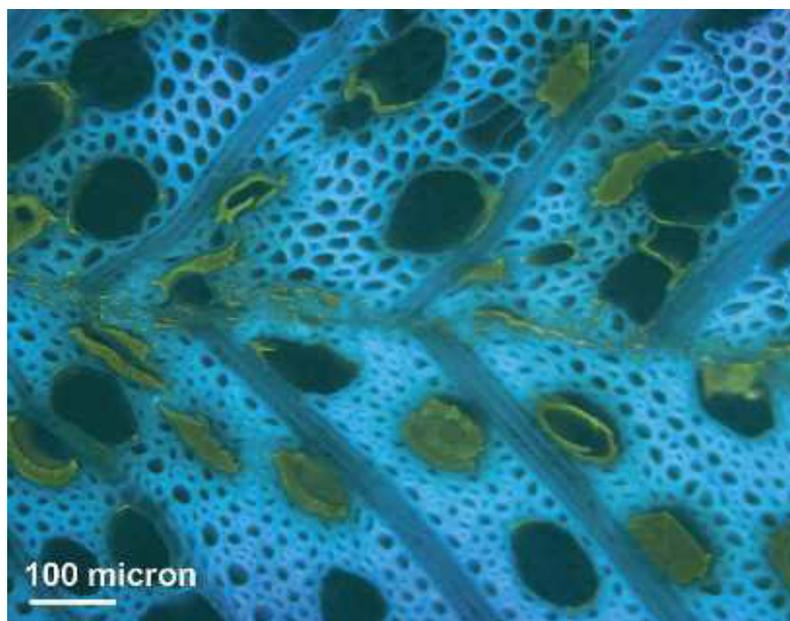
Figure 12. Photomicrograph of a PF bondline in yellow poplar using epifluorescence and stained with 0.5% toluidine blue O. Transverse view of horizontal bondline. Brown areas are resin. Filter set 360-nm/400-nm/420-nm (Zhang 2002)
