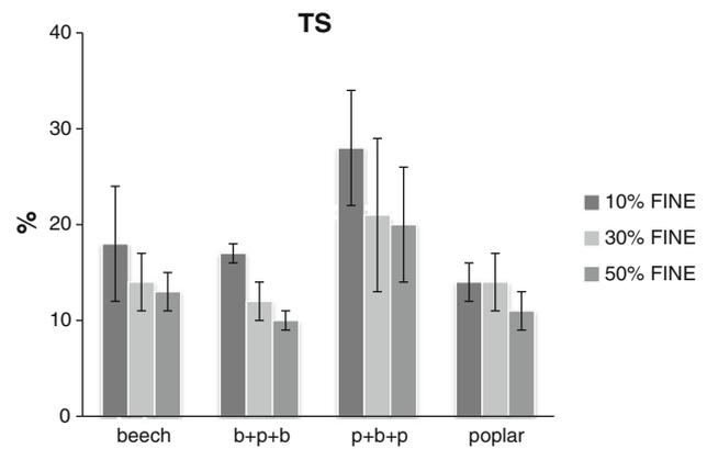
**Fig. 6** Average thickness swelling of fine core layers of 16 mm OSB. *b* beech, *p* poplar
