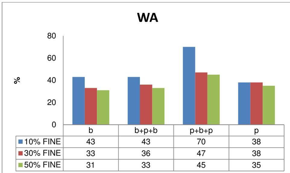
Figure 50. Average water absorption of fines core layers of 16 mm OSB
