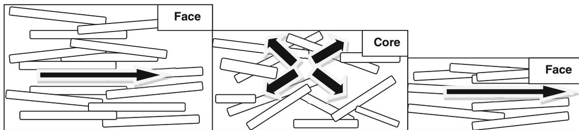
**Fig. 2** Schematic OSB mat of this research
