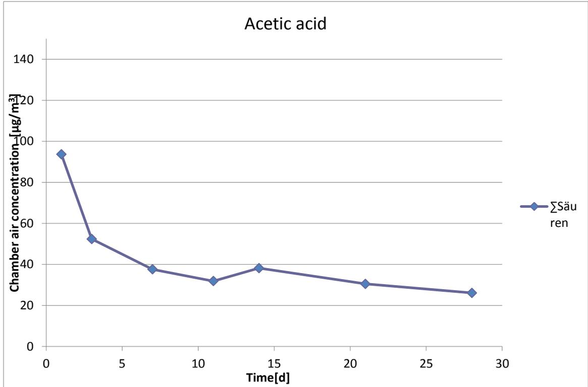
Figure 63. Acetic acid emission rate of poplar OSB during 28 days of testing
