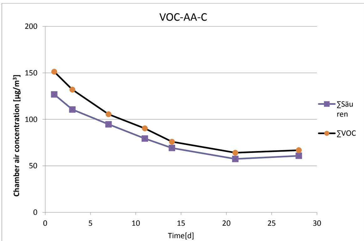
Figure 60. Total emission rate of beech OSB during 28 days of testing
