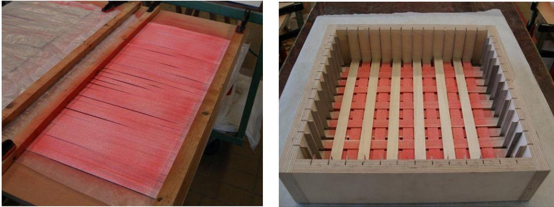
Figure 32. Fixed veneer strips by gluing with UF resin (left) and setting frame with UF resin glue-coated veneer strips (right) [Source: Leleicke 2012]
