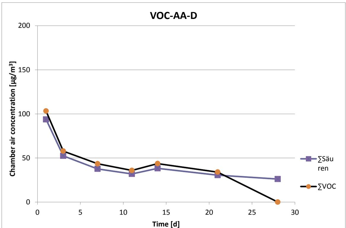
Figure 62. Total emission rate of poplar OSB during 28 days of testing
