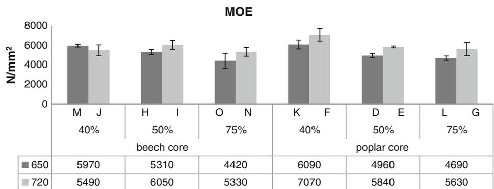
This study observed the same trend in highest MOE for panels manufactured from 60 % beech strands in faces. The highest and lowest values of MOE were 7,066 and 4,415 N/mm<sup>2</sup> for panels F and N, respectively (Fig. 4).
