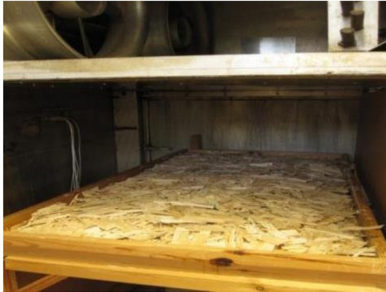
Figure 18. Kiln dryer
