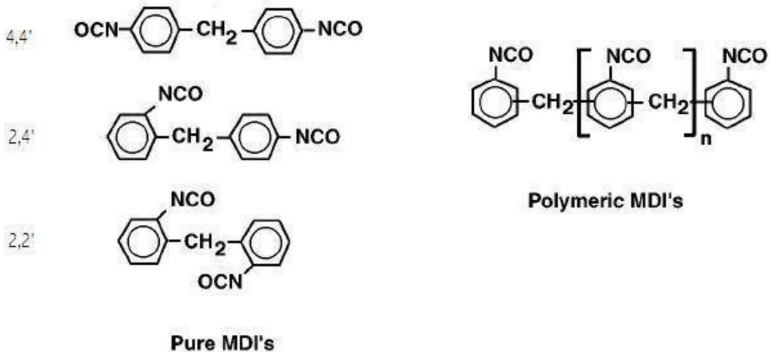
Figure 9. Pure MDI (Dow ISONATE™ and PAPI™ Pure, Modified and Polymeric MDI Handling & Storage Guide – Oct 2009)
