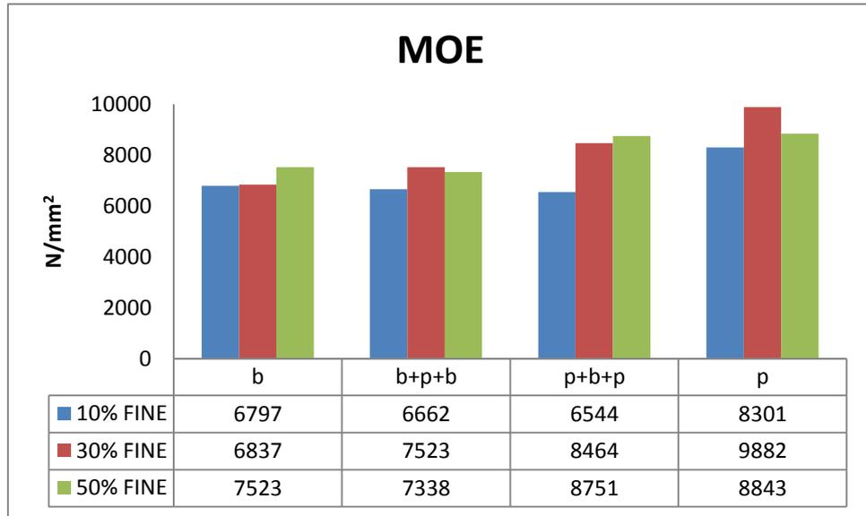
Figure 47. Average MOE of fines core layers of 16 mm OSB
