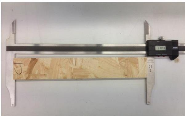
Figure 24. Length, width, and thickness measurement
