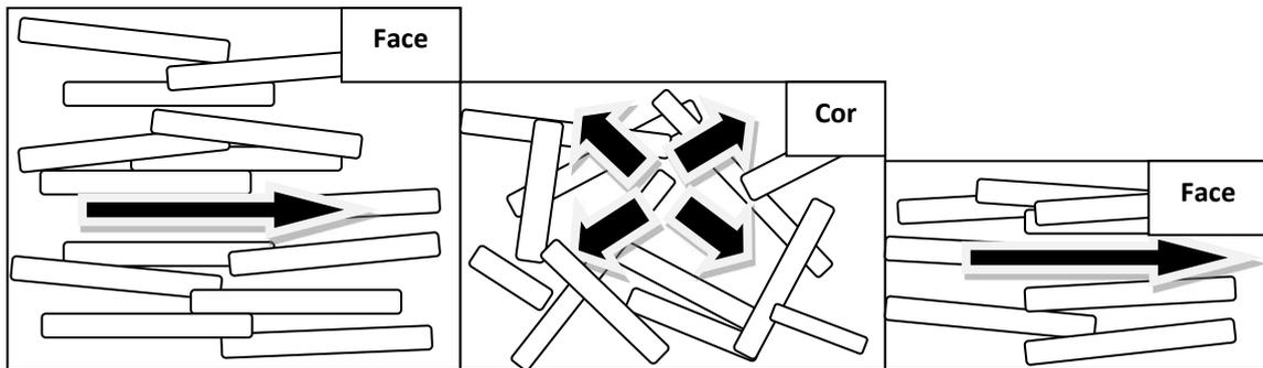
Figure 2. A schematic OSB layers
