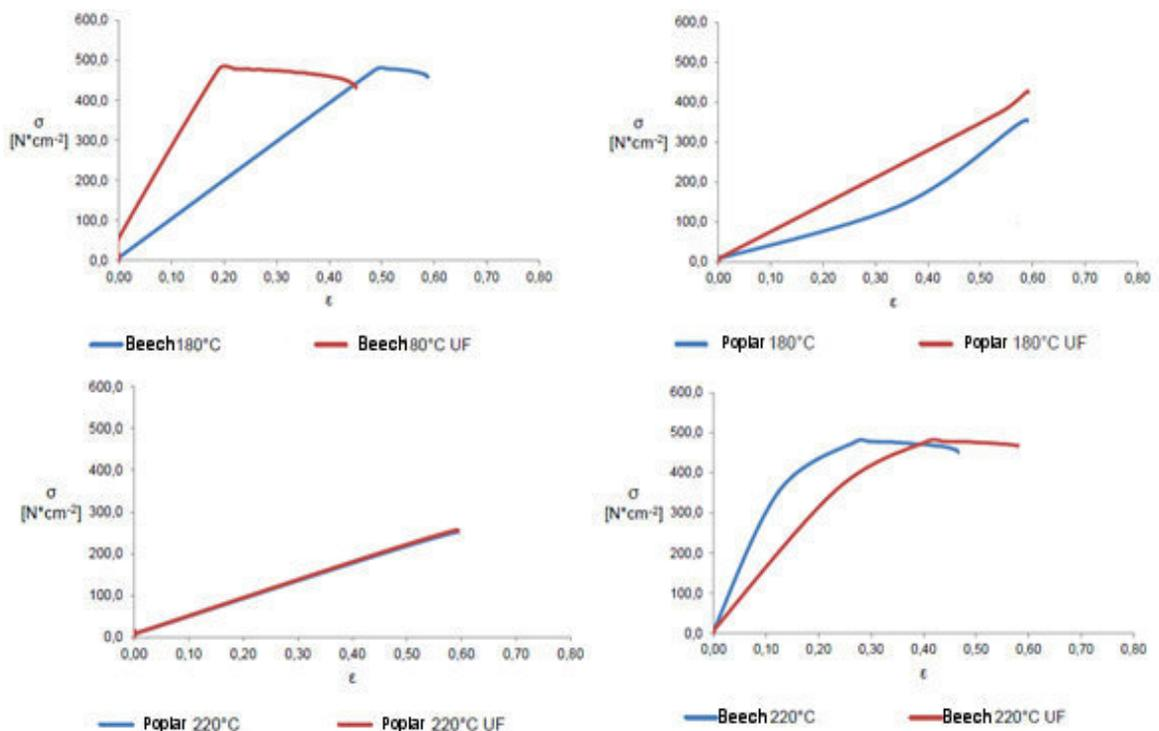
Figure 55. Stress strain diagrams of the densification experiments
