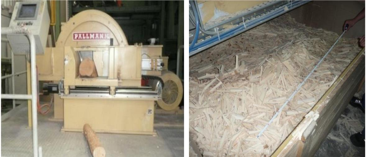
Figure 15. Knife ring flaker (left) and beech strands (right)
