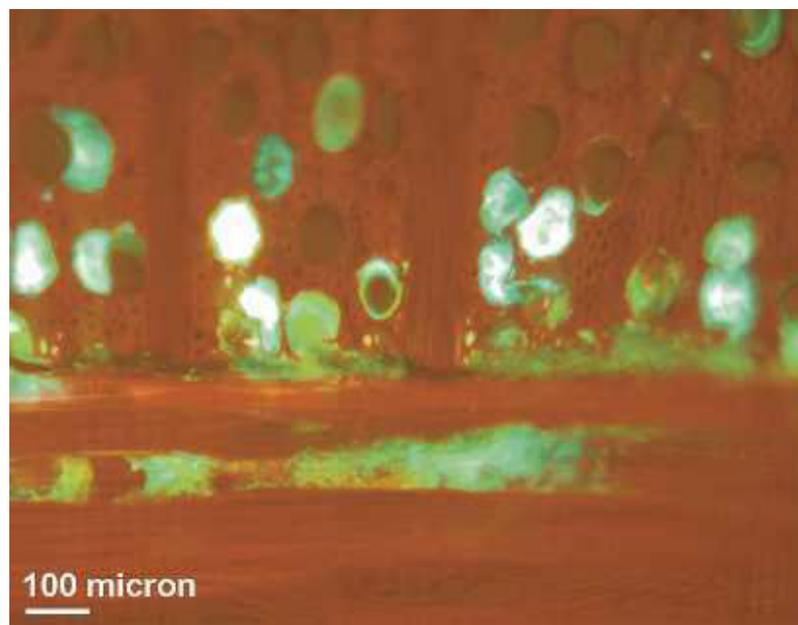
Figure10. Photomicrograph of a UF bondline in beech as viewed using epifluorescence and stained with 0.5 % safranin O. Upper lamina is transverse surface, lower lamina is radial surface. Bright areas are resin. Filter set 360-nm/400- nm/420-nm (Sernek et al. 1999)
