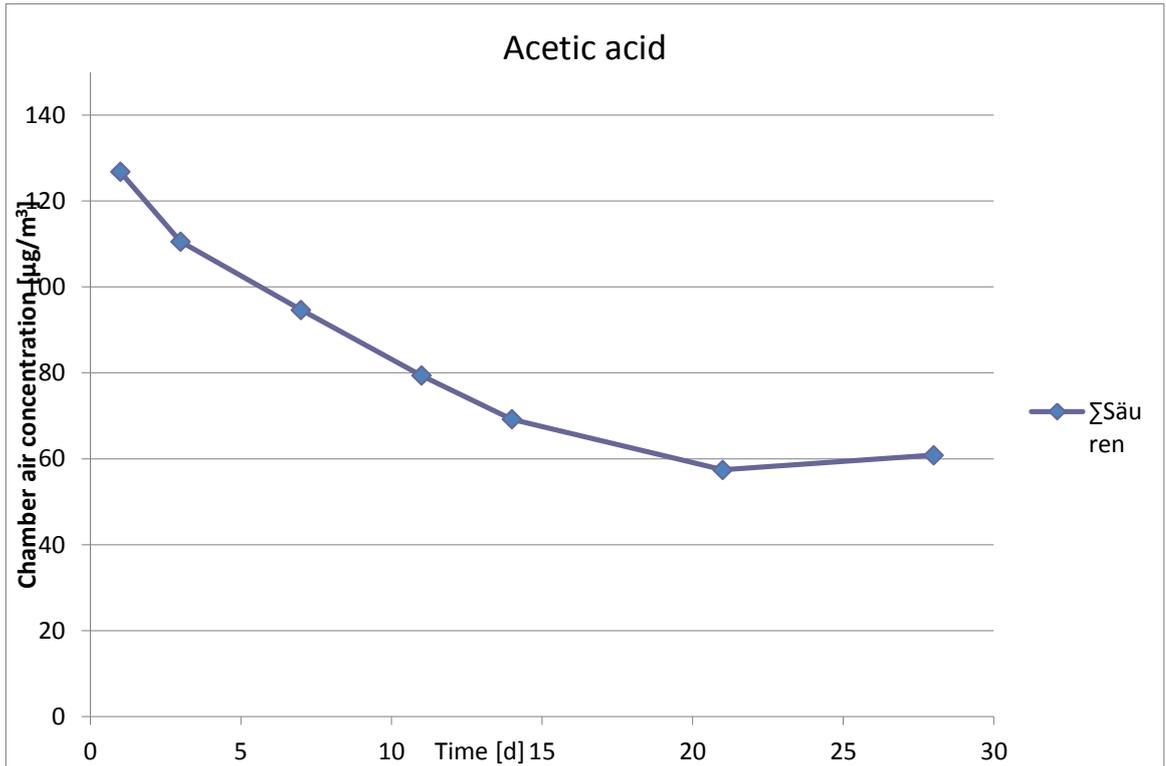
Figure 61. Acetic acid emission rate of beech OSB during 28 days of testing
