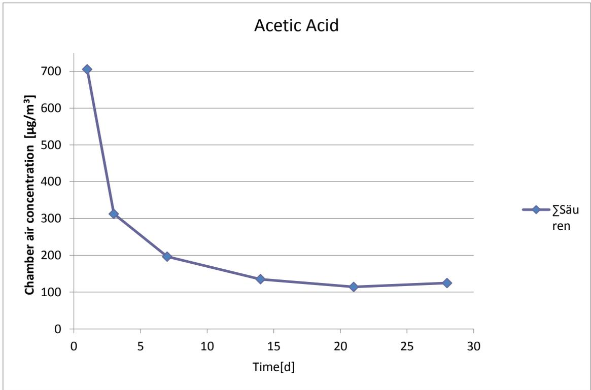
Figure 57. Acetic acid emission rate of solid beech during 28 days of testing
