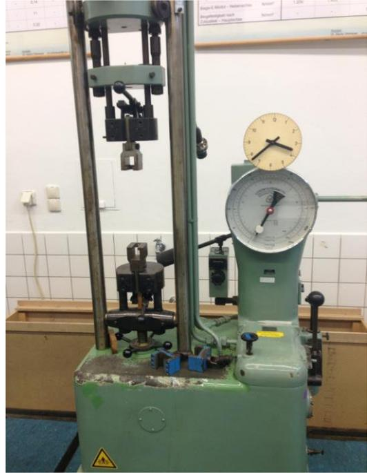
Figure 25. MOR & MOE (left) and IB (right) test
