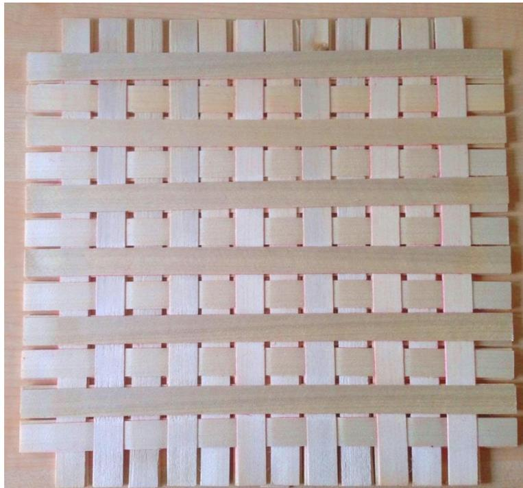
Figure 31. Mat veneer strips before compaction (mat B)
