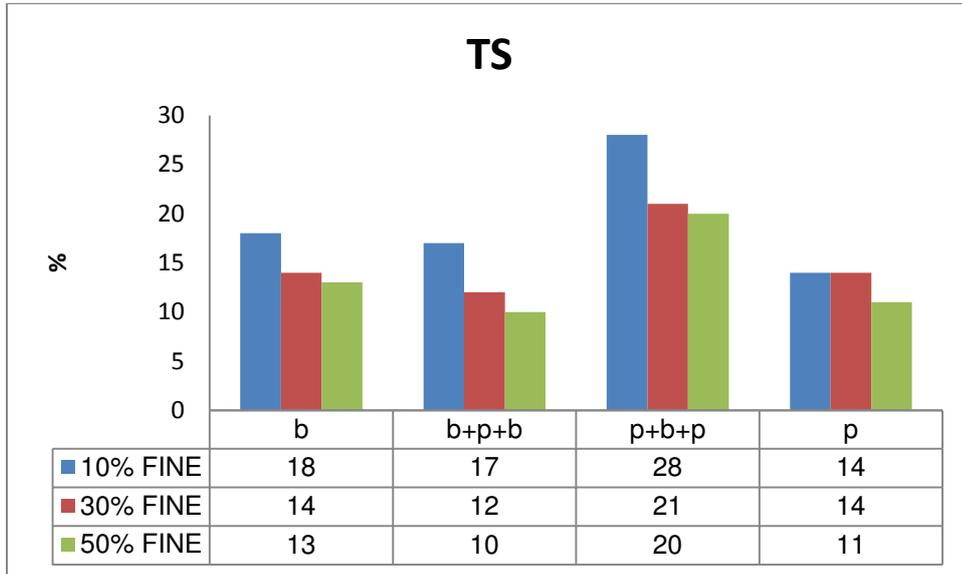
Figure 49. Average thickness swelling of fines core layers of 16 mm OSB
