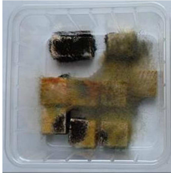
Figure 2. Naturally infection of untreated oil palm wood samples by air-borne moulds. Plastic jar with each three palm wood samples from bottom, middle and top part of the trunk. Within each part each one sample from inner, middle and outer trunk area. One Scots pine control. 75x75mm (96 x 96 DPI)
