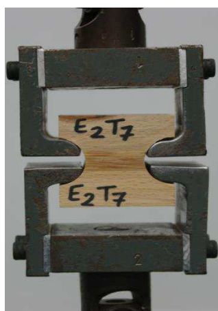
Figure 36. Apparatus to measure tension perpendicular to grain
