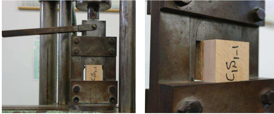
Figure 34. Apparatus to measure shear parallel to grain
