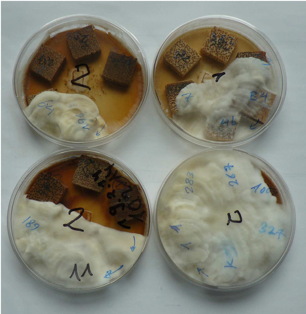
Figure 3. Examples of growth of Pleurotus ostreatus on the control (at dish bottom) and acid-treated palm wood samples. In each Petri dish from bottom clockwise: control sample and samples dipped in solution of 5 and 10% acetic acid as well as 5 and 10% propionic acid. 780x800mm (72 x 72 DPI)
