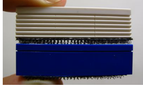
(b) LEGO bricks with hook structure at the bottom used for radiators (upper) and windows (lower)
