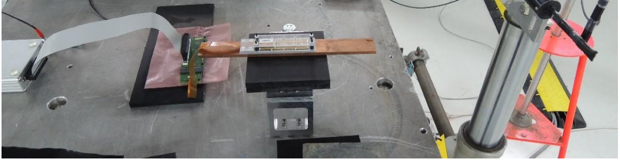
Figure D.1: Detector and trigger setup for in-plane tracking measurements. One CMS pixel module (center) is triggered by two scintillators in coincidence (top right) and readout out by the DTB (left). From [265].
