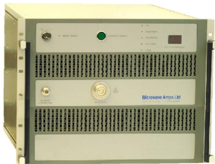
Figure 2.7: Compact rack-mountable solid state amplifier
