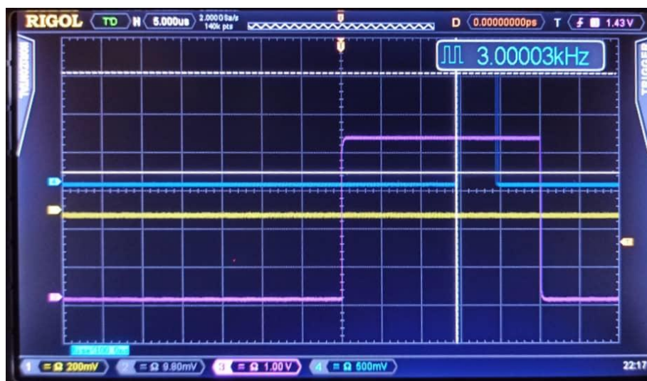
Figure 7.31: Overlapping the RF amplifier burst signal (pink) with the SDG signal for amplified laser pulses (blue) on a scope.
