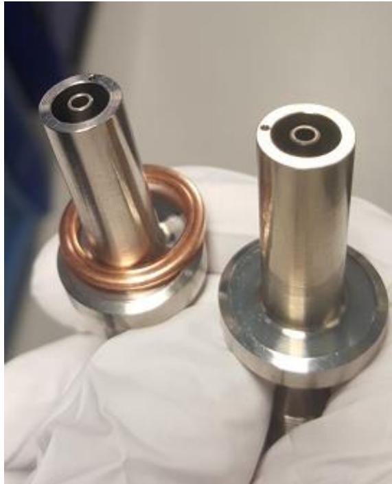
Figure 3.23: Visual inspection of the feedthroughs of the couplers after the conditioning.
