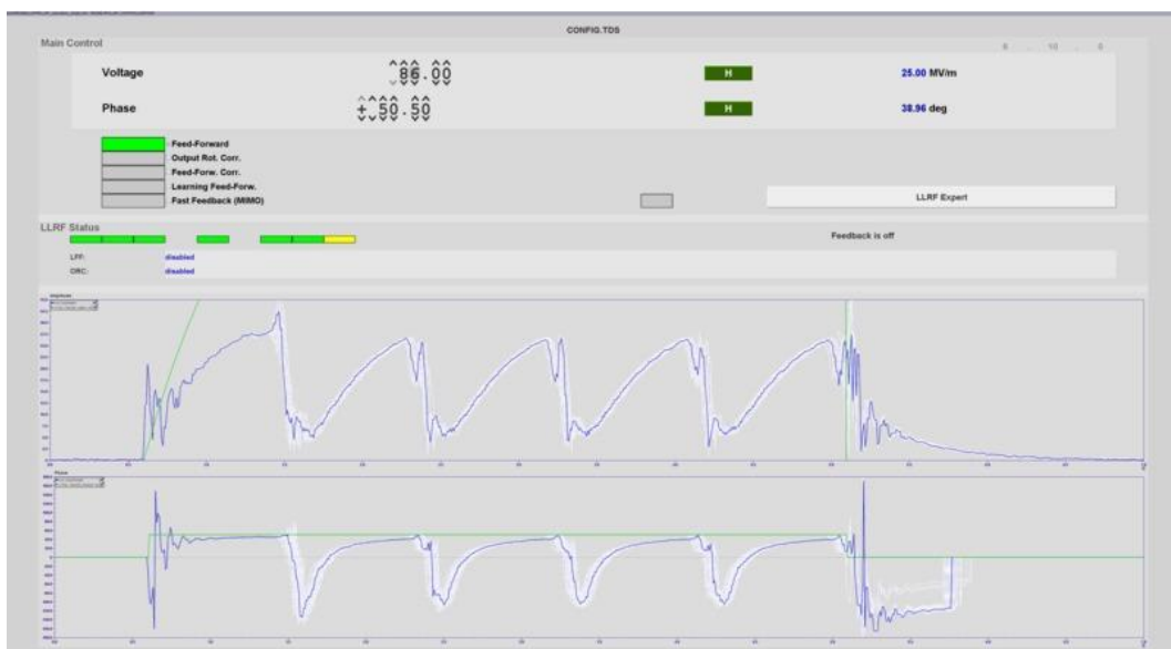
Figure 3.14: Observation of multipacing with 5 cycles at input power of 2.1 kW
