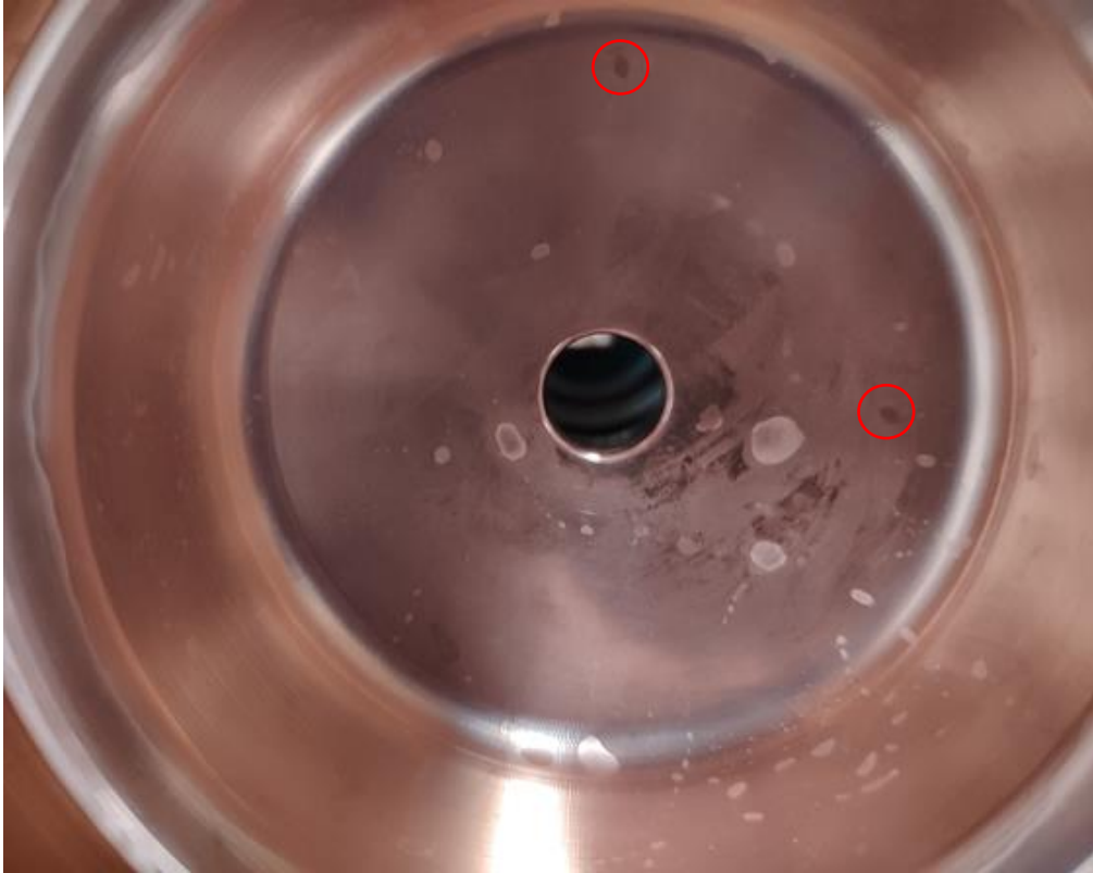
Figure 3.22: Visual inspection of the anode part of the gun after the conditioning.
