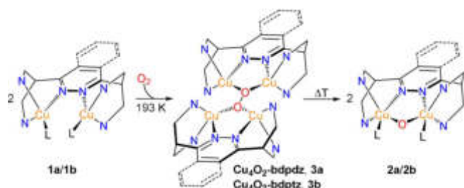
Scheme 2. Formation of the Cu 2 O core via homolytic O–O bond cleavage of the tetranuclear, mixed-valent \mu_4 -peroxo species ( Cu 4 O 2 ). The pyridine rings have been omitted for clarity and simplified by the N-donor atoms.
