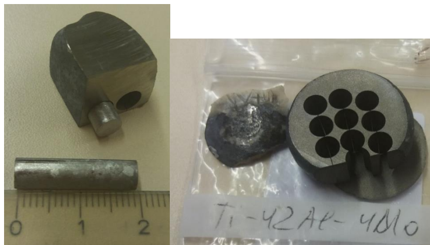
Figure 11 Parts of the button used for neutron diffraction analysis (cylinders) and other methods for the first and the second sample sets
