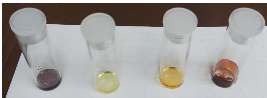
Figure 34. Crude product with 33 wt% S, first collected drops of distillate, last collected drops of distillate, obtained product after vacuum distillation (from left to right).
