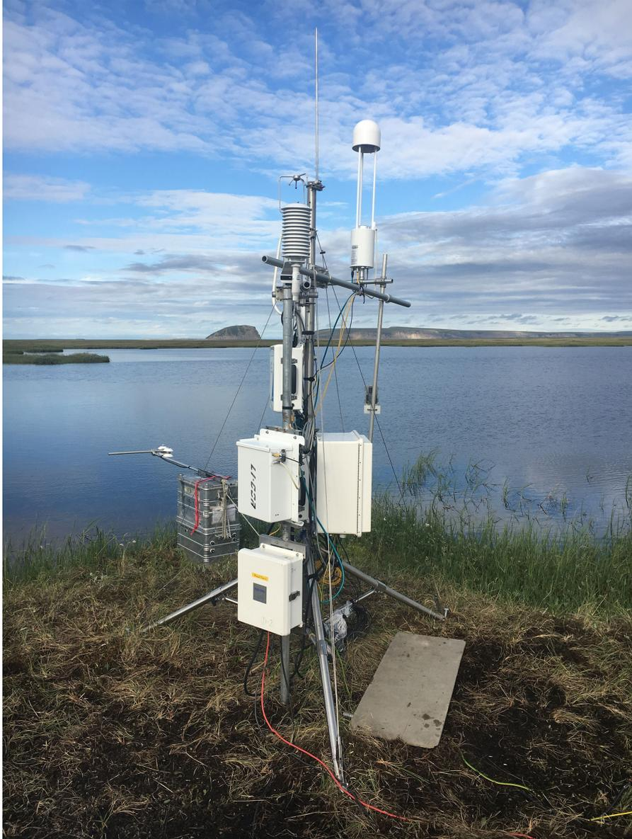
Figure 17: Picture of the eddy covariance tower with the merged polygonal pond in the background. Picture taken on 11 July 2019 by Zoé Rehder.
