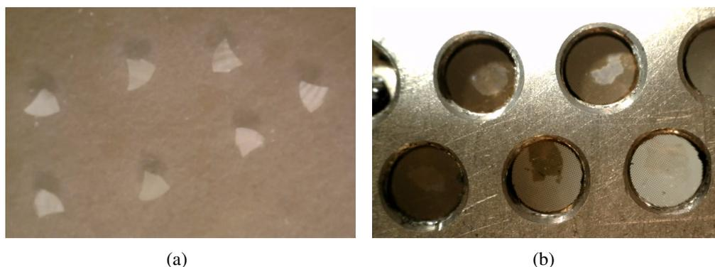
**Figure 2.20:** Ultrathin samples of butyl-dithienylethene (a) for transient absorption spectroscopy on a UVFS substrate and (b) for ultrafast electron diffraction on copper TEM meshes inside the sample holder.
