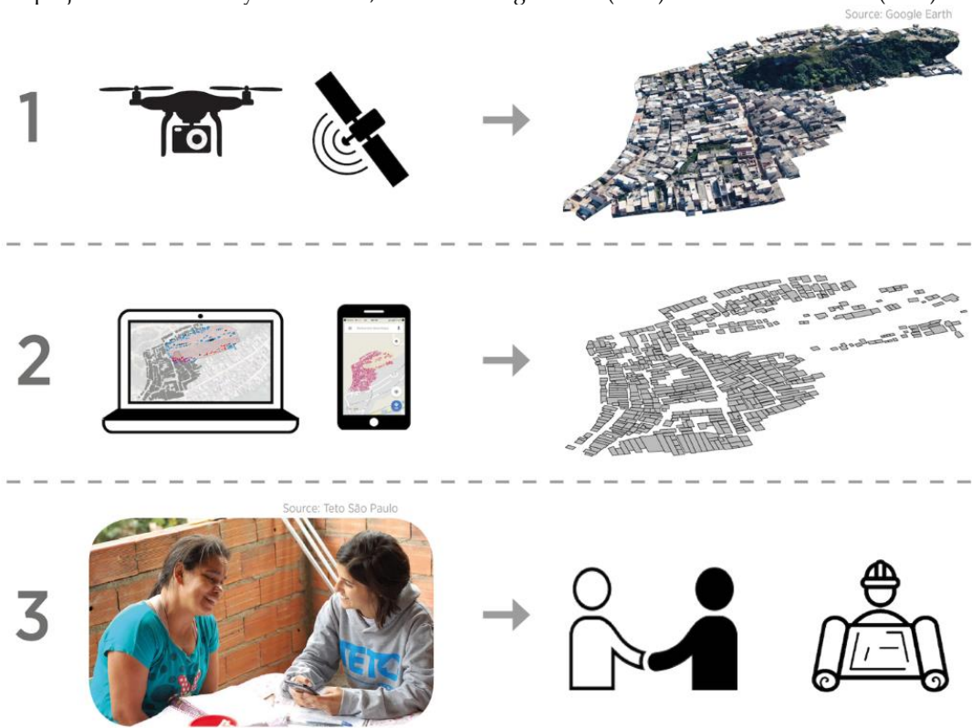
Figure 6-2. Teto's mapping process, step-by-step (1) acquiring drone or satellite imagery; (2) digitizing building footprints, with on-site verifications using Google My Maps; (3) validating GI data to obtain geographic information that may support upgrading projects. Elaborated by the authors, based on Google Earth (2018) and Pessoa Colombo (2019).
