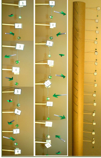
Figure 4.3: Magnetomechanical model of [53]. The magnets are not connected by a wire. They are hanging each on their own soft, nonmagnetic filament and they are coupled via magnetostatics only. The hole is larger than the diameter of the filament and magnets may rotate without screwing it. Left: Stable spin helix with modulation vector q = (3/2)\pi/14 . Right: General view of the model. Silver and green colors represent the north and the south poles, respectively.
