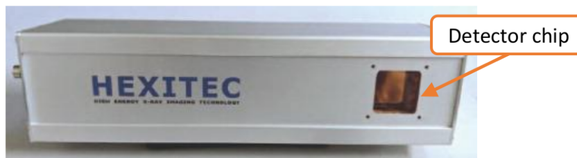
Figure 9.10: Photograph on the HEXITEC detector system. On the right side of the image, the pixelated semiconductor chip is visible. The remainder is mostly made up of electronics. The detector chip was covered by a 1.5 mm thick aluminium plate during the X-ray spectrum measurements to further attenuate the X-ray flux. Photograph taken from [180] .
