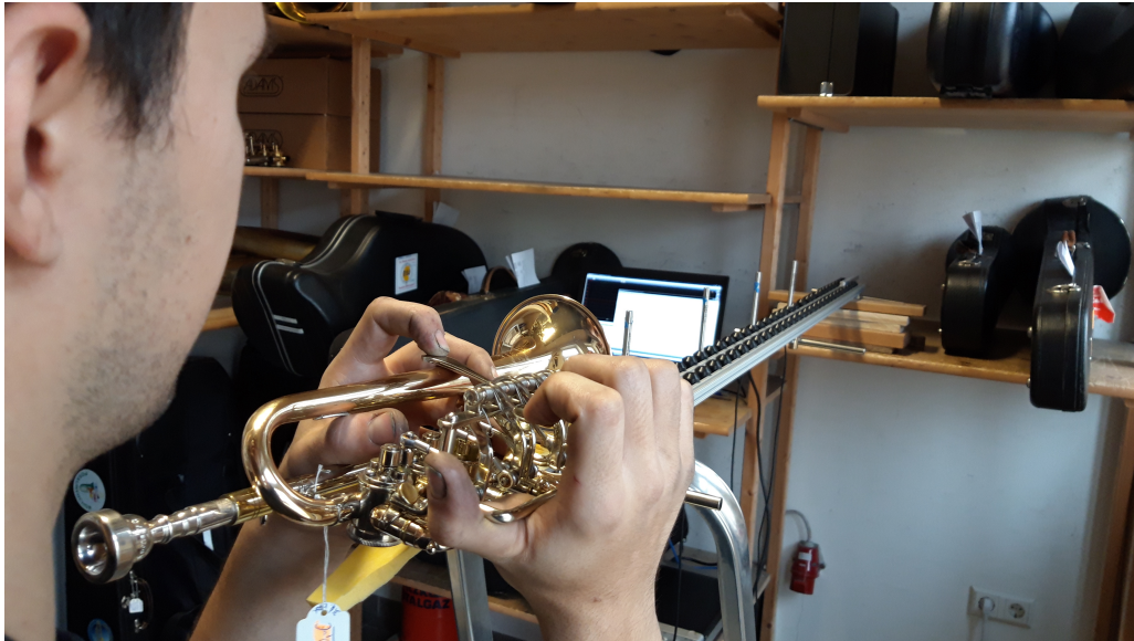
Figure 5.3: High speed measurement set-up. To record the propagation speed of the initial pressure waves leaving the instrument a linear microphone array with four iSEMcon EMX-7150 microphones at relative positions y_{mic1} = 0.0 mm, y_{mic2} = 243.0 mm, y_{mic3} = 486.0 mm and y_{mic4} = 729.0 mm is used. The microphones are mounted at a bar of aluminum. The signals were recorded with a sampling rate of f_s = 500 kHz.
