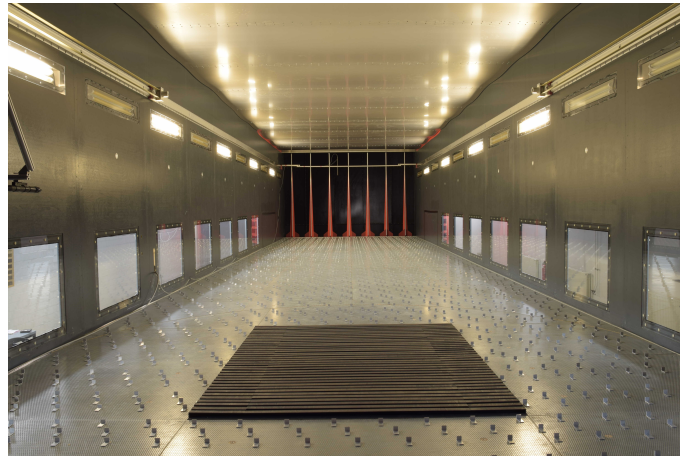
Figure 4.1: Upwind view of the experimental setup in the test section of WOTAN . Foreground: Rectangular black area with balcony-shaped roughness elements at s_b = 5 m. Background: Upstream area with the red spires and floor roughness used for generating an artificial thickened, turbulent, equilibrium boundary-layer flow.
