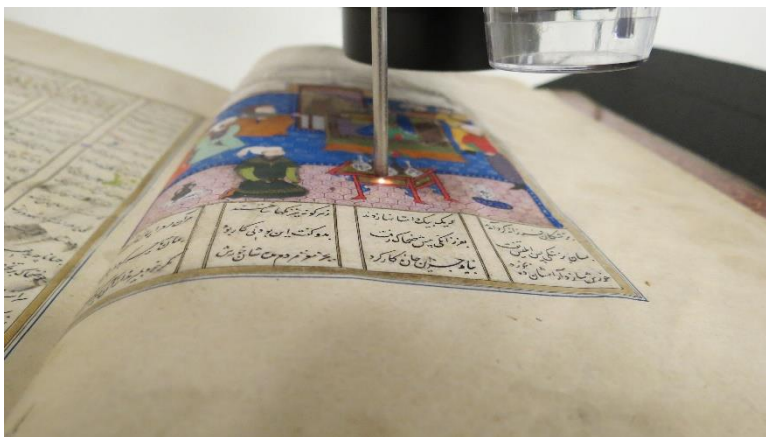
Figure 3-6: Setup for technical FORS instrument equipped with fiber-optic
