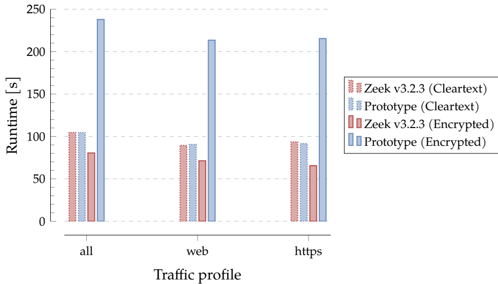
FIGURE 4.3: Results: Decryption overhead for passive TLS decryption
