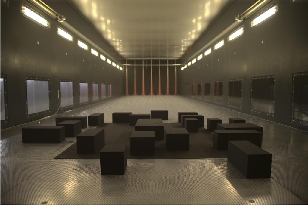
Figure 4.4: Idealized industrial park model in the wind tunnel. View from the back of the wind tunnel towards to the model along the x-axis.
