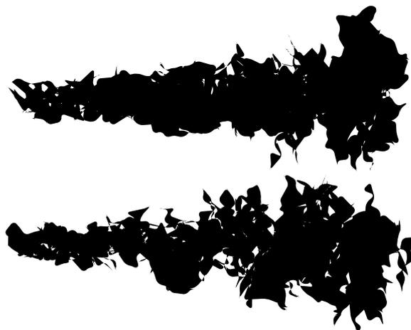
Figure 3.1: Exemplary illustration of two turbulent jets. The upper jet has a higher Reynolds number compared to the lower jet. The large scale structure does not change significantly as long as the jet is turbulent. Adapted and reproduced from Snyder (1981).
