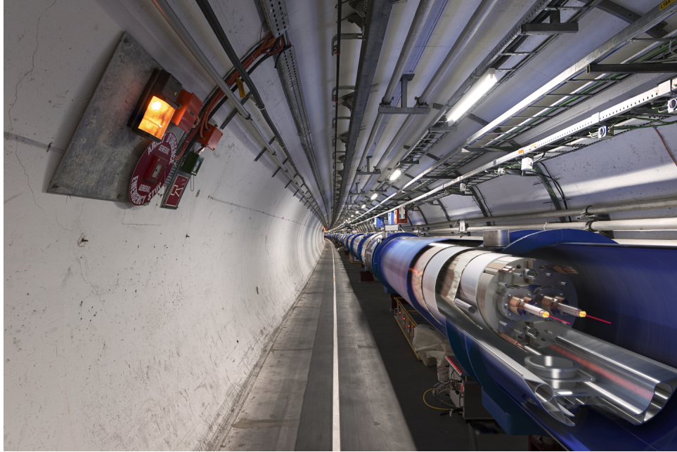
Figure 3.1: Picture of the LHC with a 3D cutaway artist's impression. The proton beams are accelerated in opposite directions along the red lines. Figure taken from Ref. [145].
