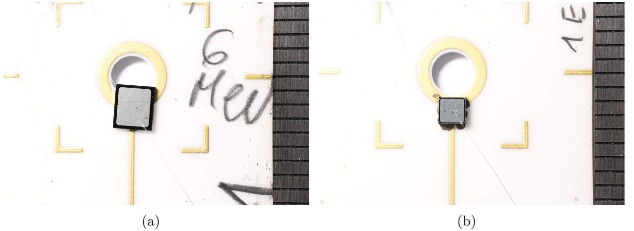
Figure 7.1: Overview of the diodes irradiated by 5.5 MeV electron. (a) Epitaxial, (b) Czochralski.
