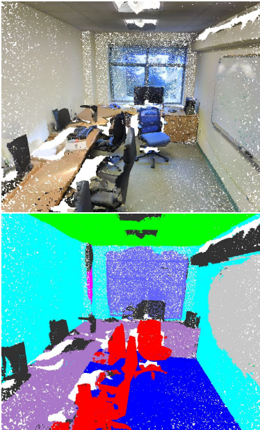
Figure 6.2: Qualitative performance of PointNet on 3D scene segmentation using the S3DIS dataset [179]. The top plot shows the input point cloud, representing an office scene in 3D. The bottom plot shows the PointNet model, trained to classify each point as one of 13 categories. Taken from [173].
