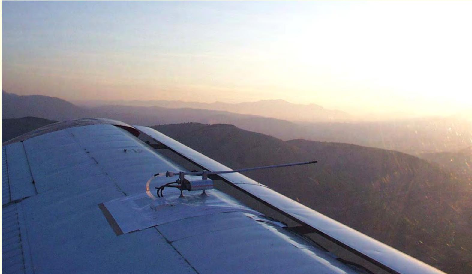
**Figure 6** Probes of the online system for meteorological measurements mounted on the left wing.
