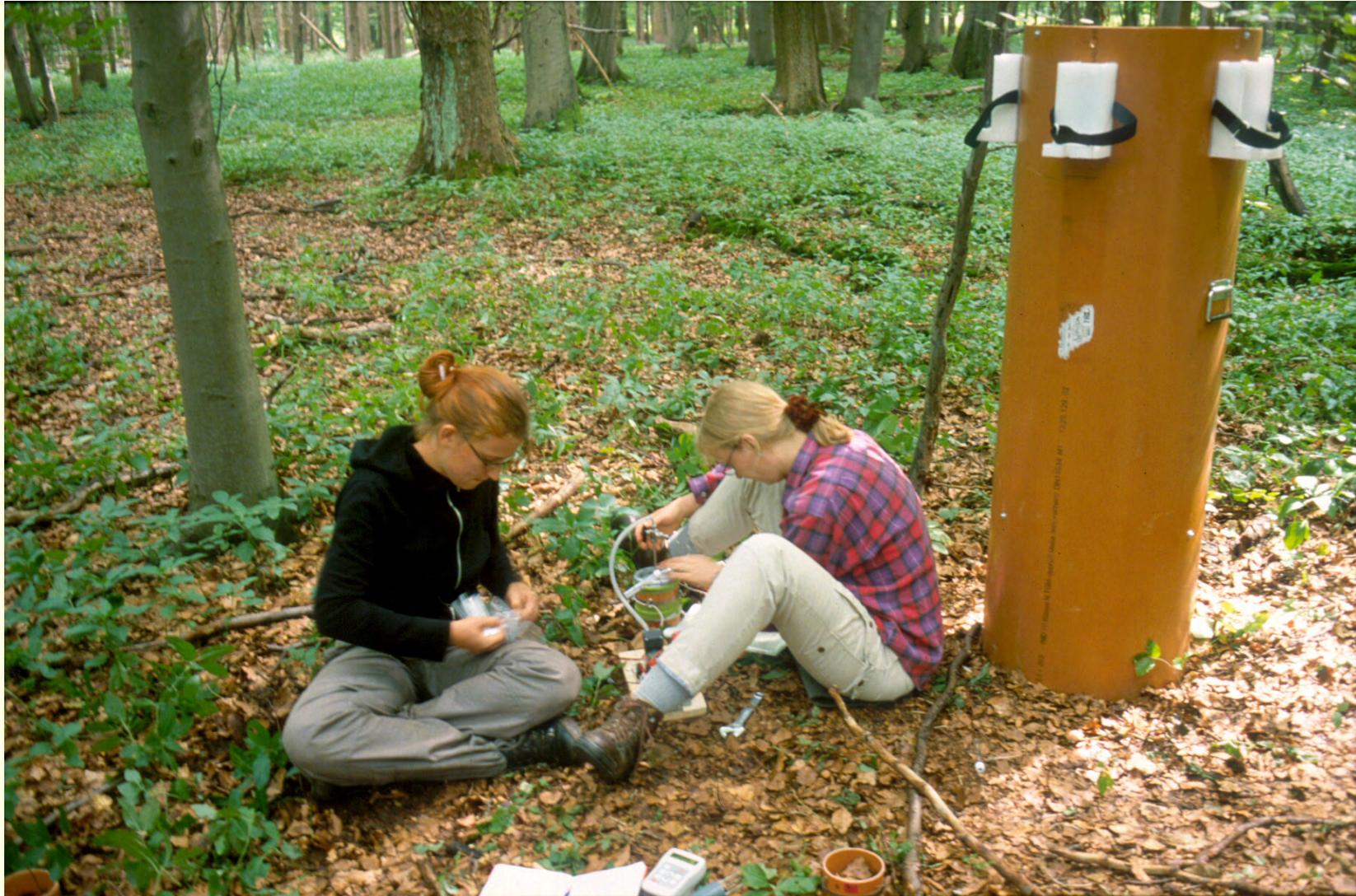
**Figure 8** Soil respiration sampling from cylindric sections as visible in the front (right hand site of the sketch book). Filling of small cuvettes for isotopic analyses. Inside the big ,chimney' flask sampling profiles of respired air were carried out.
