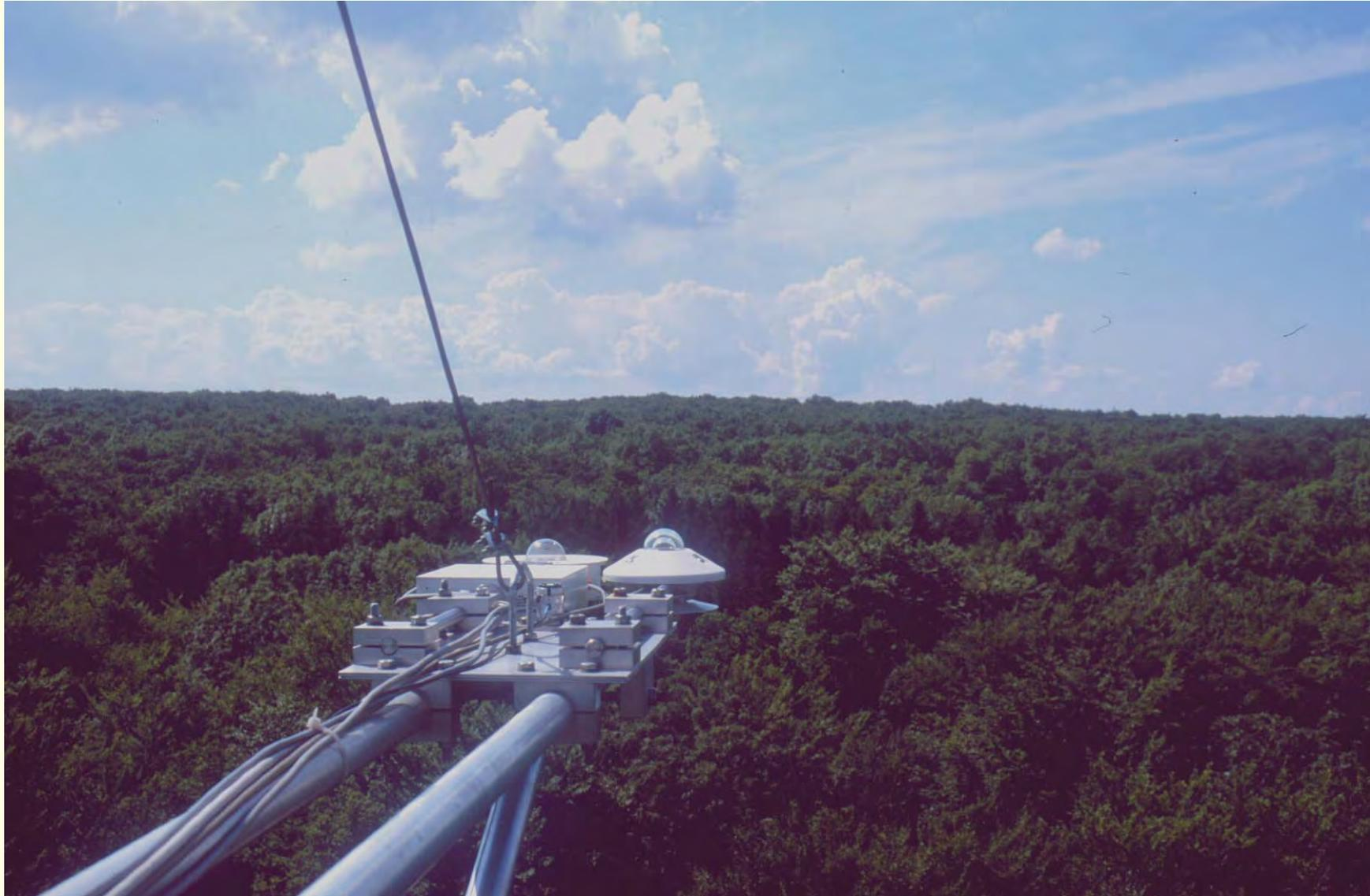
**Figure 4** View from the Hainich Tower over the canopy to the South. Placed on the boom are the sensors for radiation measurements.
