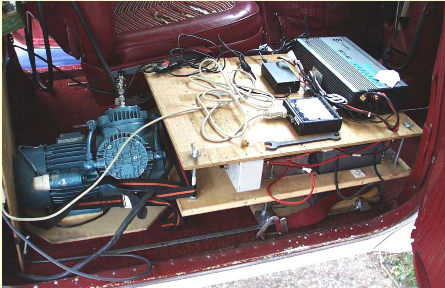
**Figure 6** Pump and power supply installed at the copilots place inside the cabin.
