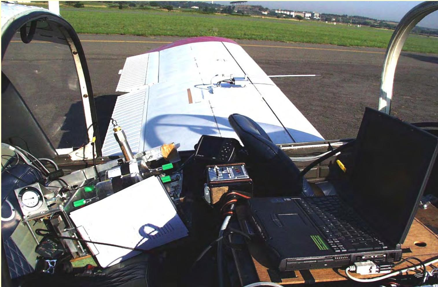
**Figure 7** FlightSamplingUnit, GPS (on the barrier between front and rear seat), switch box of the continuous measurement system in front of the GPS. Laptop for system controlling and data recording – during the flight fixed on the operators thigh. Sample flasks are stored in the rear of the cabin Recognizable are on the left wing the mounted sensors for air temperature and humidity, dynamic and static pressure and the compass module.
