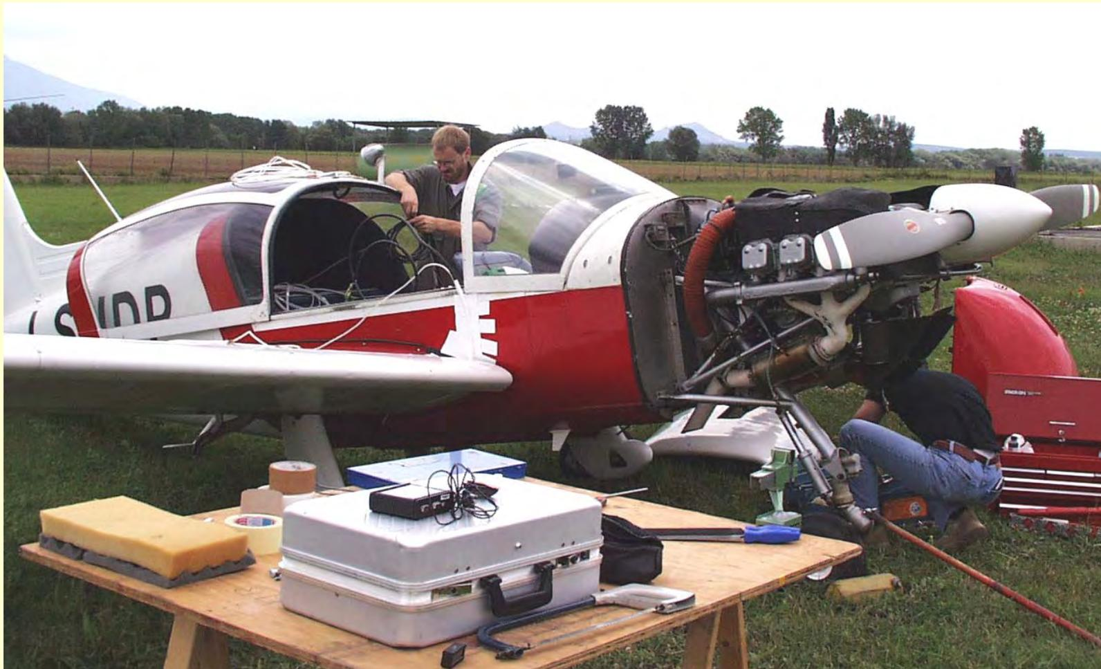
**Figure 5** Installation of the flight equipment at the Montorotondo Airfield in Italy. Location of the air inlet was on the right wing tip. The tube is covered by the wing nose, becoming visible at the white taped section. Aircraft is a Morane Socata.
