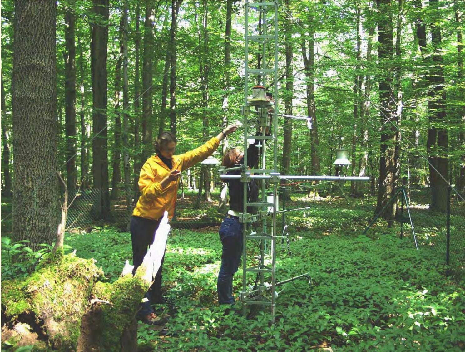
**Figure 5** Small mast for near ground measurements close to the main tower (height 3.0 m).
