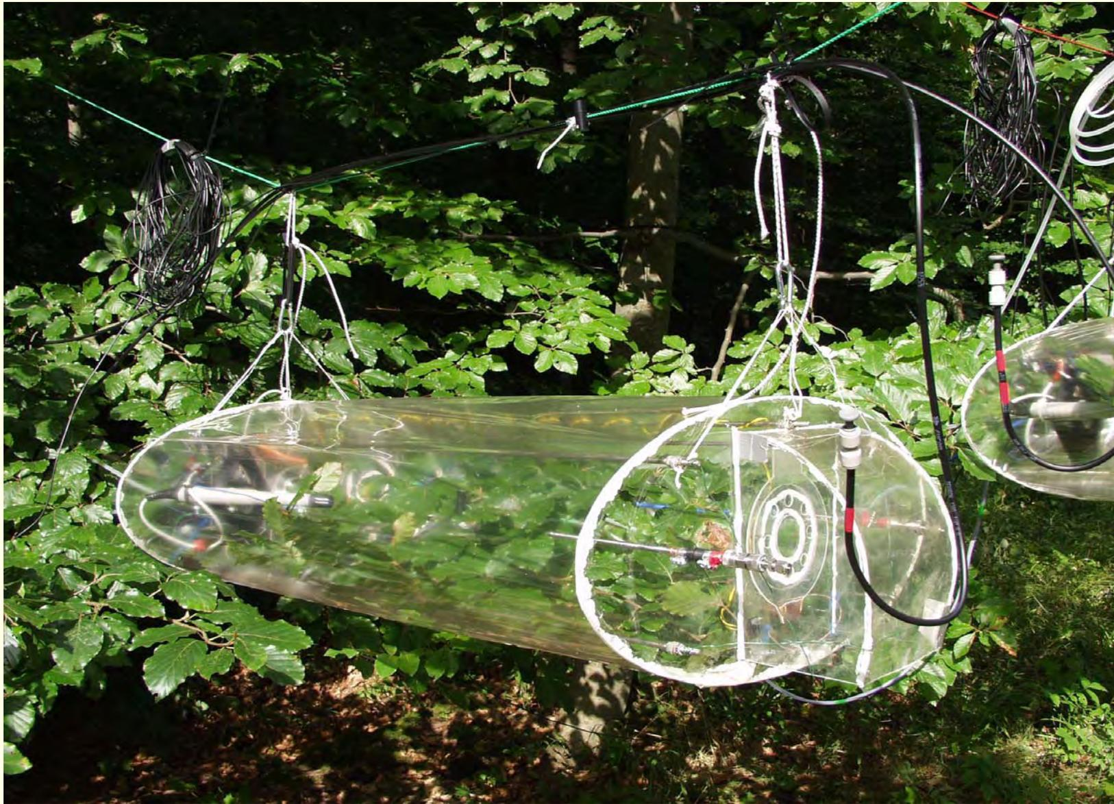
**Figure 6** Branch bags with enclosed beech twig for direct sampling of air characterized by assimilation and respiration.
