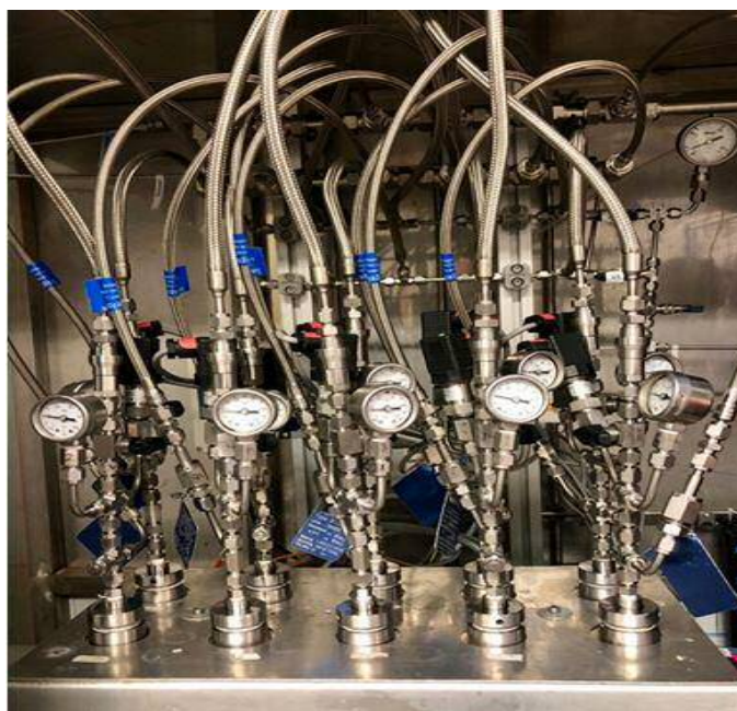
Figure 6.2 Ten-fold parallel reaction system used for hydroprocessing reactions.
