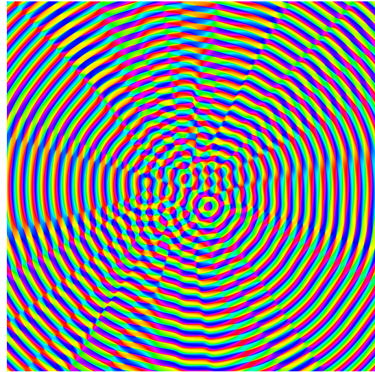
(b) Phases of the simulated diffraction using only the Fourier components of the object that lie on the Ewald sphere.
