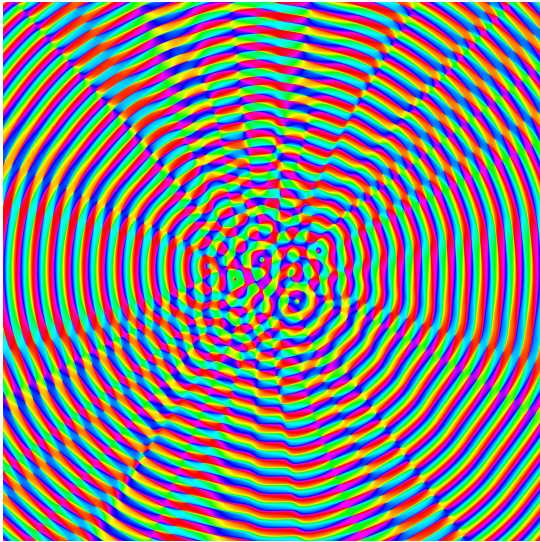
(a) Phases of the simulated diffraction using a discretization of Green's function.
