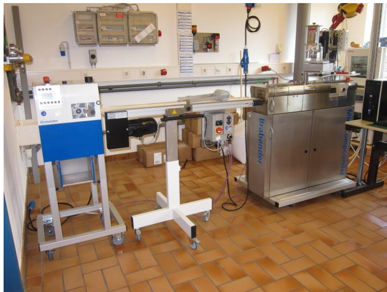
Figure 18: Twin-screw compounding extruder used in this work.
