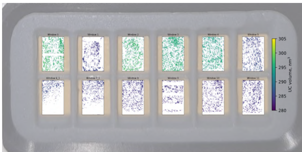
Figure 5.17: Spatial distribution of unit cell volume of FAKP crystals on the chip with 6 \times 2 compartments, each 4.22 \times 4.8 \text{ mm}^2 in size.
