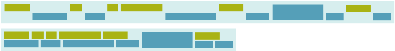
Fig. 2: Comparison between sequential (first row) and parallel execution. The coloring denotes different resources used for some task (for example different robots which manipulate or localize). Note that the start of the tasks is not necessarily synchronized. The block, spanning two rows, is a task, which requires both instances of some resource, for example during handover both arms are blocked.
