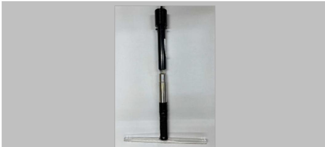
Figure 2: Oxygen sensor. The oxygen sensor (O<sub>2</sub> Microsensor OX-500-007533, flowcell, glass, UNISENSE, Denmark) has a "T-shape". The glass tube on the one end of the sensor was integrated into the tubing of the experimental setup. The wire on the other end of the sensor is connected with the UNISENSE amplifier.
