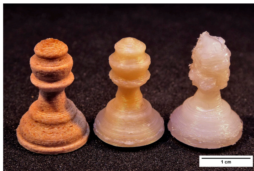
Figure 9. Three-dimensional printed models: filament used on the left pawn is Woodfill, HDPE for the middle and CNF-PSA/HDPE composite for the right one.
