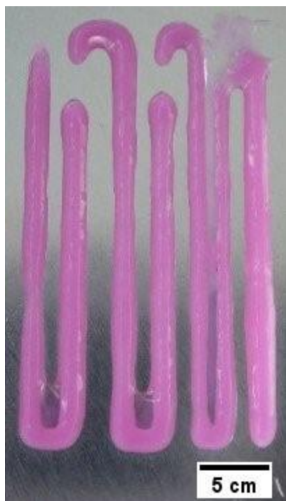
Figure S6. Picture of the printed model of a pattern with gradually increasing distances (0,5 and 1 mm between strands) using CNF-g-UPY/UPY-DEGEEA composite
