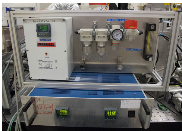
Figure 3.8: The mass flow controller, the upper device, regulates the flow rate of gas. The Eurotherm controller, which is located at the bottom of the mass flow controller, can be used to control the temperature of each gas blower.
