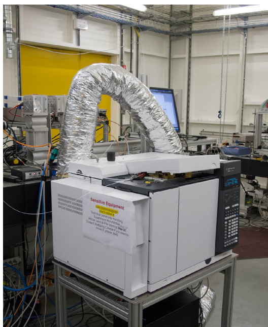
Figure 3.12: GC was used to separate and analyze the chemical components of the sample online in the XANES tomography imaging measurement of this work.
