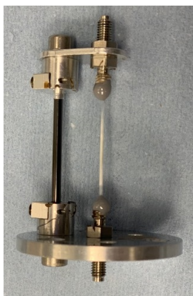
Figure 6.1: Filled quartz capillary with the catalyst powder of \text{MoO}_3/\text{Al}_2\text{O}_3 was glued on the sample holder. The capillary inlet was located at the top of the setup.
