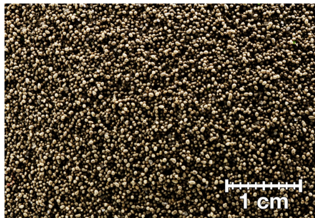
Figure 2.25: Macro photo of expanded glass.
