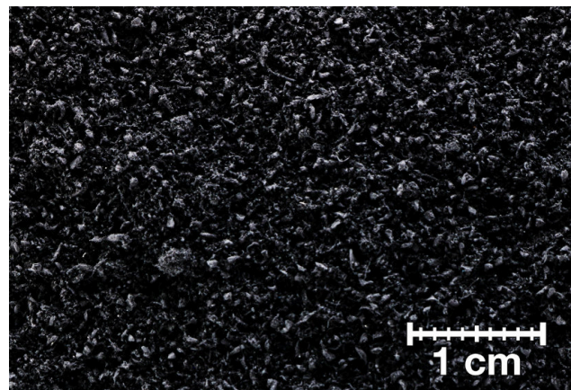
Figure 2.34: Macro photo of rubber granulate black.
