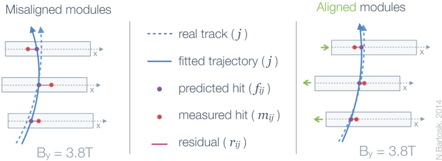
Figure A.1: Schematic representation of the fitted track prediction according to the alignment of the tracker modules. The local hit positions are constant, and only the global position will change according to the alignment of the modules. The increase in the track-hit residuals due to misaligned modules is also illustrated [222].
