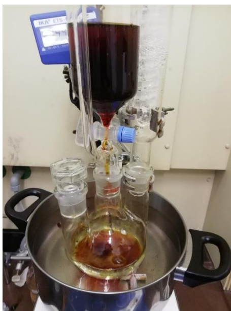
Figure S40. The cooled solution of \text{H}_9\text{PV}_{14}\text{O}_{42} in water is dropped into the boiling solution of \text{MoO}_3 and \text{H}_3\text{PO}_4 in water.
