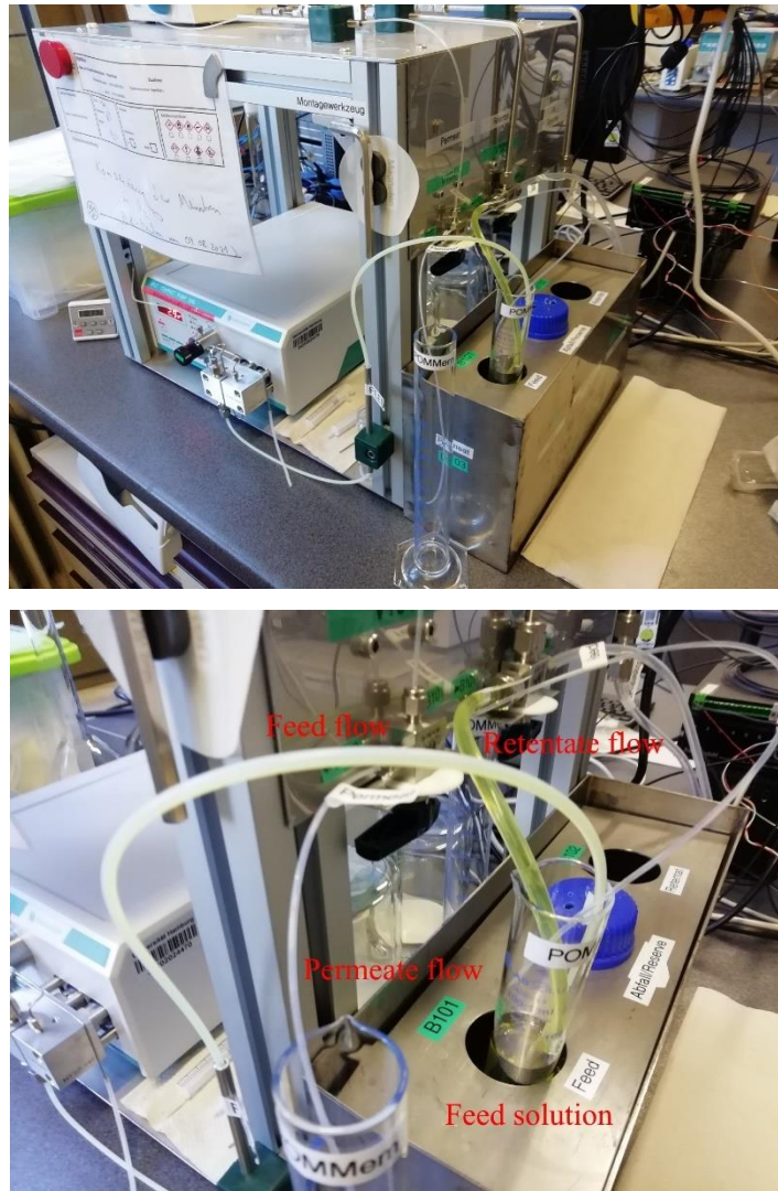
Figure S49: Membrane plant used for nanofiltration to remove salts from the POM solution. Here: purification of \text{NaKPNb}_3\text{Mo} (yellow solution).
