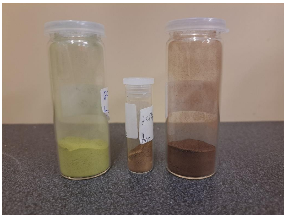
Figure S4: HPCo x Mo POMs synthesized in this work. From left to the right: x = 1, 2 and 3 . The more Co(II) in the Keggin structure the darker the POM.
