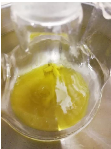
Figure S39. After the suspension of \text{MoO}_3 and \text{H}_3\text{PO}_4 in water has been heated to boiling point for about one hour, a yellow, clear solution is formed.
