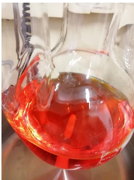
Figure S42. During the synthesis of \text{H}_8[\text{PVMnMo}_{10}\text{O}_{40}] a red, clear reaction solution is formed.
