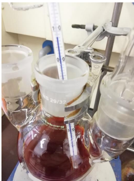
Figure S37. Solution of \text{H}_6\text{V}_{10}\text{O}_{28} in water after adding \text{V}_2\text{O}_5 , hydrogen peroxide and water.
