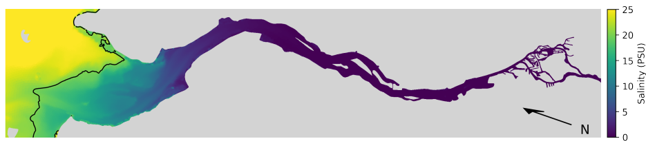
Figure 4.8: Salinity map of the Elbe estuary, with Hamburg's port area (as shown in Fig. 2.14) at the bottom right. Salinity is averaged across depths and over the whole year. The 20 PSU isohaline is marked with a black line. Note that this plotted area has been extended downstream compared to Fig. 2.18. Also note that the color map has been capped at 25 PSU for better visibility in low-salinity areas.
