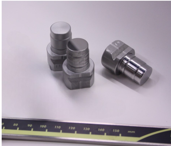
Figure 4.1: Photograph of polished standard Mo plugs that are used as substrate in the production system for the deposition process.
