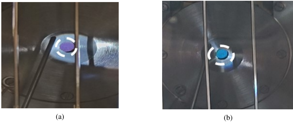
Figure 4.57: Colors of photocathodes after the deposition (a) 137.3, i.e., thin cathode (violet in color), and (b) 137.2, i.e., thick cathode (blue in color). Since the cathode is placed behind the masking system, the active photoemissive area is highlighted by the white dashed circle for both cathodes.
