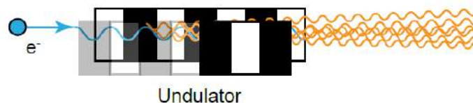
Figure 2.8: Radiation from insertion device: an undulator.
