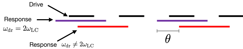
Figure 2.9: Sketch of the phase relation between the drive and the response of the limit cycle for subharmonic entrainment. Solid lines denote times when \cos(\omega t) > 0 . \theta denotes the phase difference entrained limit cycle if \omega_{\text{dr}} = 2\omega_{\text{LC}} and the entrained limit cycle with a different driving frequency.
