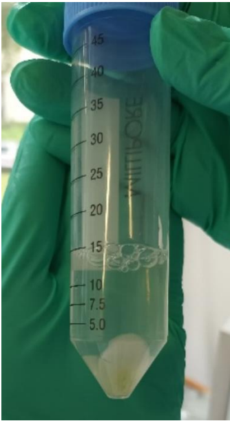
Figure S.1: Taxus baccata nuclei pellet in 50 ml tube in NIB wash buffer after last washing step with NIB.
