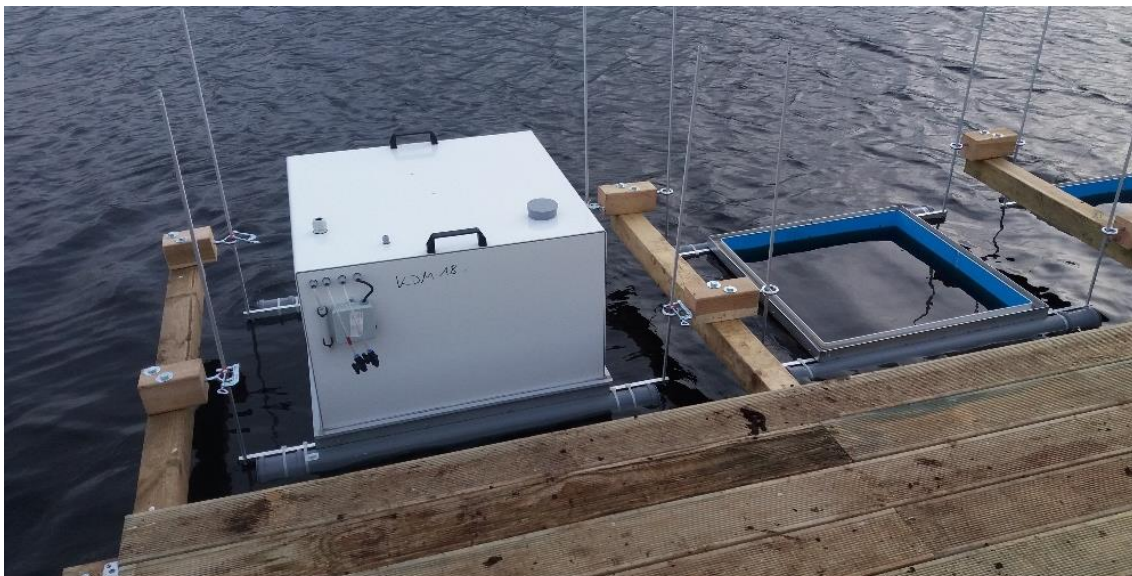
Fig. 2.8: Buoyant base and measurement chamber at the polder site at Provinzialmoor.
