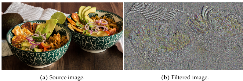
Figure 7.7: Source image and filtered output image of the image convolution task for edge kernel.
