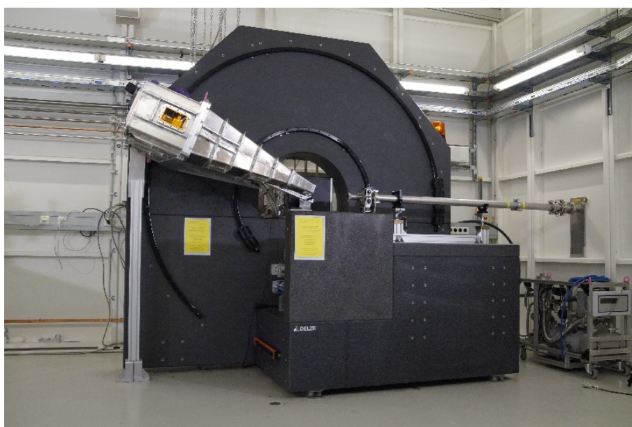
Figure 3.7: XRS setup at P01. The conically shaped aluminum tank hosts 12 Si(220) analyzers for XRS experiments. Courtesy of Kai Schlage.
