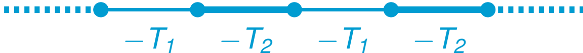
Figure 3.2: Sketch of a one-dimensional SSH model. The different electron sites (blue dots) are connected via an alternating electron hopping T_1 (weaker) and T_2 (stronger).
