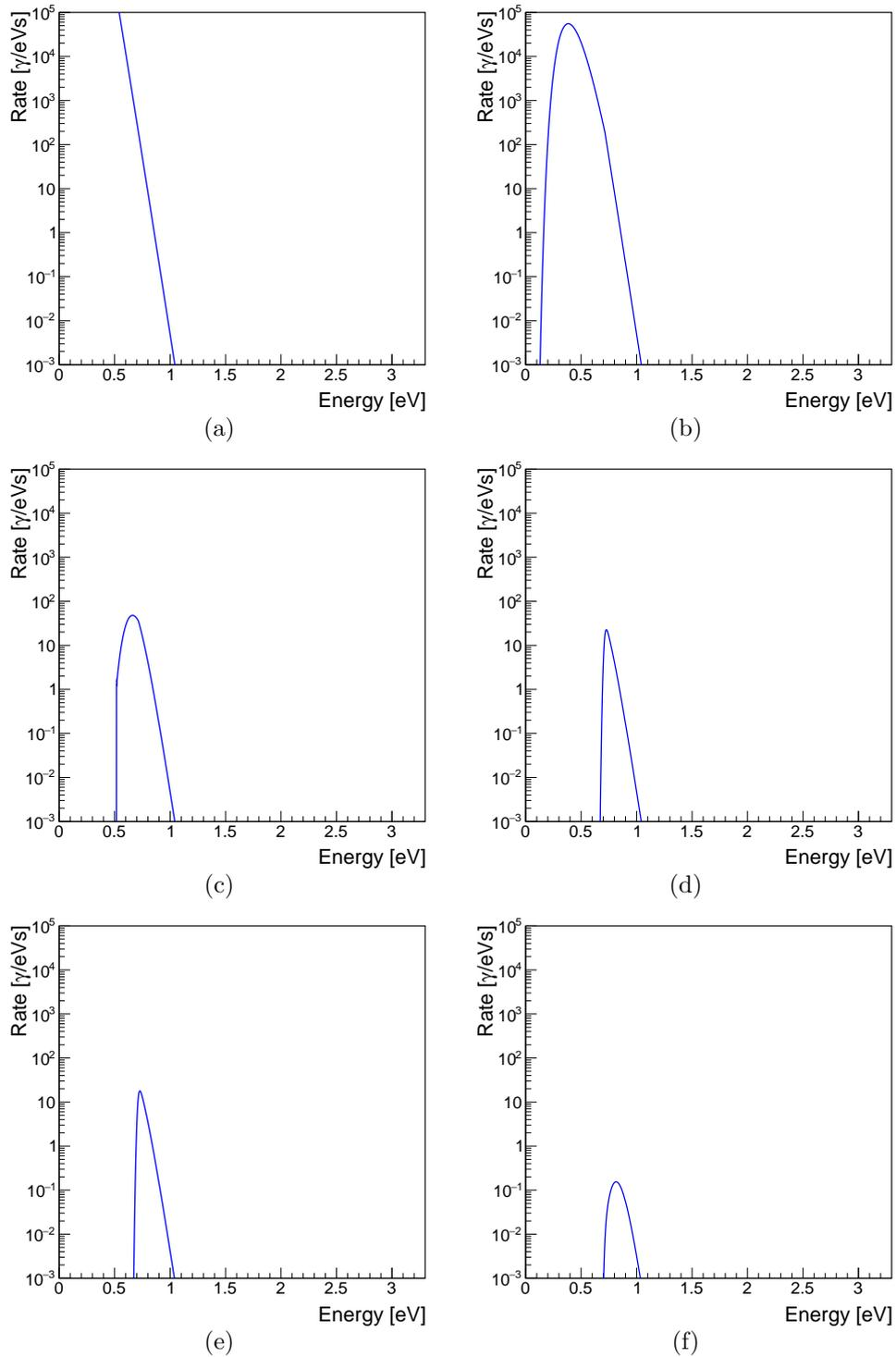
Figure 4.7: BBR spectrum computed from Eq. 4.8 including optical components step by step: (a) no components, (b) optical fiber transmission  $\eta_{\text{fiber}}$ , (c) adding curling with 4 loops with diameter  $d = 11.2$  cm  $\eta_{\text{curl1}}$ , (d) adding curling with 1/4 loops with diameter  $d = 2.5$  cm  $\eta_{\text{curl2}}$ , (e) adding the absorbance of the TES optical stack, (f) extra curling considered for the lower limit in Fig. 4.8.
