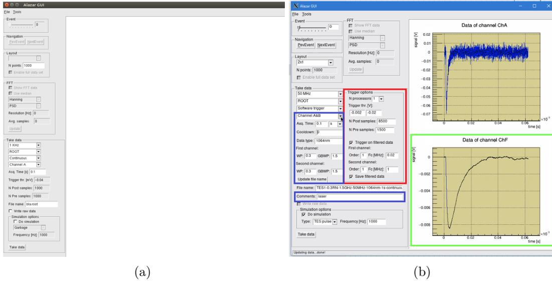
Figure D.1: AlazarGui interface (a) before and (b) after the upgrade. The section inside the blue boxes shows the new data which can be saved in the file. This includes the information on the cooldown corresponding to the data taking, a short description of the measurement setup, and the SQUIDs and the TES working parameters. The pulse inside the green box corresponds to the filtered samples used for triggering while avoiding high-frequency fluctuations.
