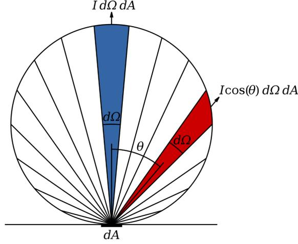
Figure 4.1: Scheme of the flux emitted in a solid angle by a Lambertian radiator. The flux depends on the angle  $\theta$  between the normal to the surface and the direction of emission [Taken from Wikimedia Commons].
