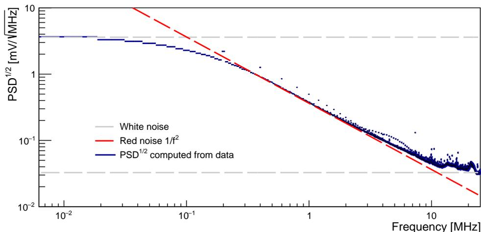
Figure 5.2: PSD of noise in data in blue. Small peaks represent the noise coming from harmonics, specifically 200 kHz harmonics. The white noise dominates at frequencies below 50 kHz and above 10 MHz. The Brownian noise ( $1/f^2$ ) dominates between 100 kHz and 10 MHz.
