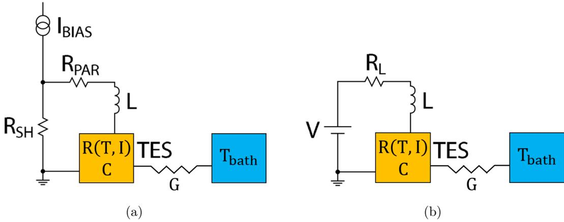
Figure 2.1: (a) Model of the electrical and thermal circuits in the TES. The TES is kept hotter than the thermal bath due to the heat produced by the Joule power and the weak thermal link, with thermal conductance  $G$  defined in section 2.1.1, with the bath. (b) Same model as before, but the electrical circuit is replaced by its Thevenin equivalent.
