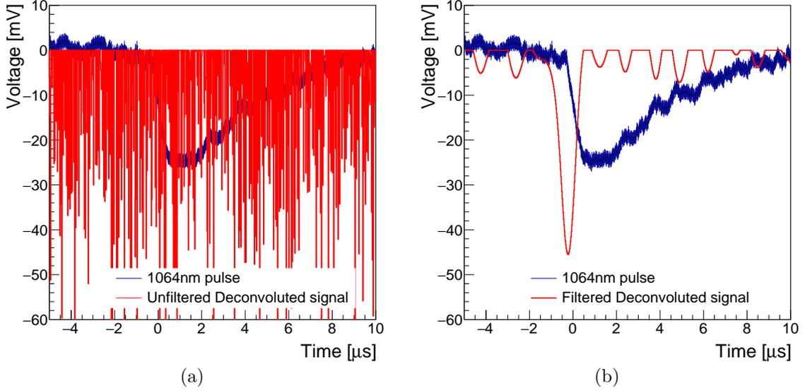
Figure 6.11: (a) A 1064 nm pulse from data and its deconvolution without filtering. No features can be distinguished in the timeline. (b) Same data but with a filter in the deconvolution at  $\sigma = 0.5$  MHz, resulting in a peak with a FWHM of  $\Delta t = 0.75$   $\mu\text{s}$
