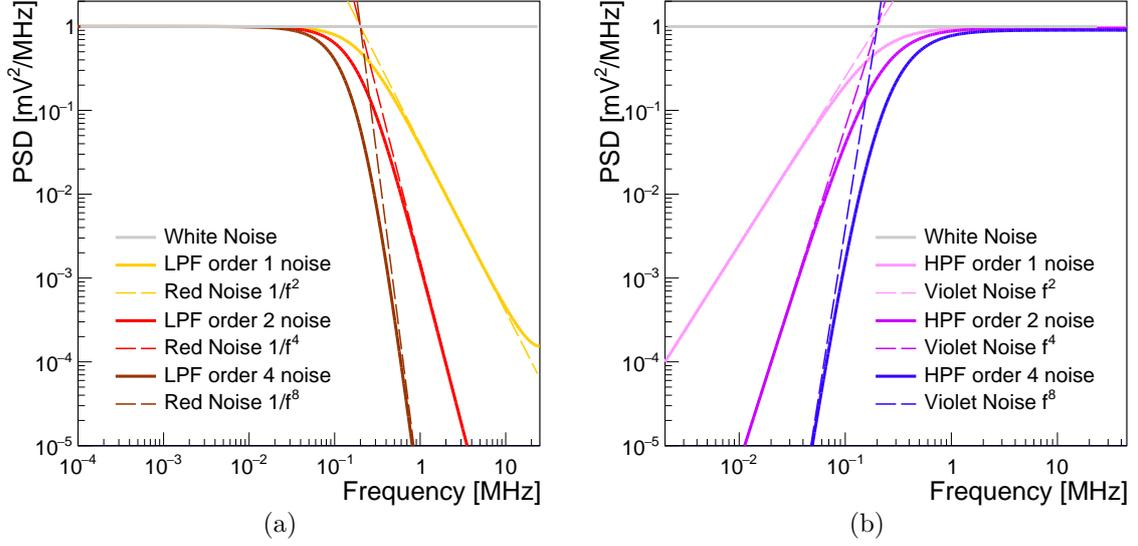
Figure 5.6: Comparison between the response of the filters and the noise. The dashed lines intercept at the cut frequency of the filters, set at 200 kHz. (a)  $n$ -order low-pass filters (LPF) against  $1/f^{2n}$  noise, (b)  $m$ -order high-pass filters (HPF) against  $f^{2m}$  noise.
