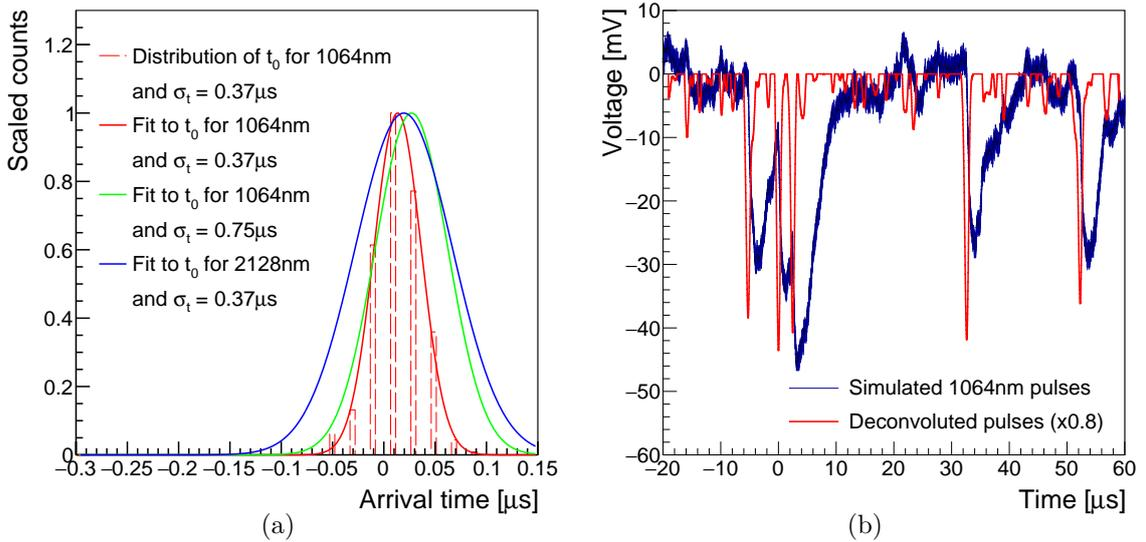
Figure 6.12: (a) Distribution of arrival time  $t_0$  for simulated samples with the start time of the signal at 0. The distribution broadens for lower energies and cut frequencies (worse time resolution). (b) Simulated pulses at a high rate. The deconvolution produces a peak per pulse. If a threshold is imposed over peaks of the noise but below the peaks of the pulses, e.g. at 20 mV, the peaks which pass the threshold can be identified as signals.
