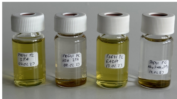
Figure 7.31: Photo of colloidal MUA-capped Pt-CdSe/CdS DRs in water in the presence of IPA, a mixture of KOH & IPA, EtOH, and a mixture of sulfide & sulfite (from left to right). While the NPs are colloiddally stable for weeks in the presence of the alcoholic EDAs, they precipitate within hours after introducing the hydroxide & alcohol mixture or the sulfide & sulfite mixture.
