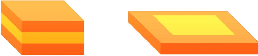
**Figure 6: A core-shell NPL (left) and a core-crown NPL (right), where the core material is depicted in yellow and the shell/crown in orange. The left image is recreated from literature,<sup>32</sup> and the right image is also recreated from literature.<sup>34</sup>**
