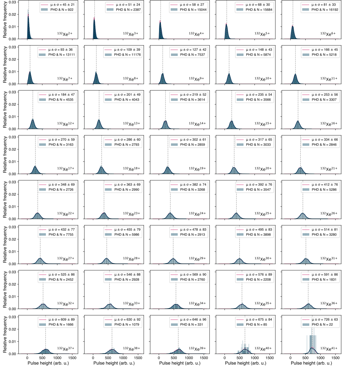
Figure A.3: Peak fitting of individual PHDs using a gamma distribution function to extract the mean.
