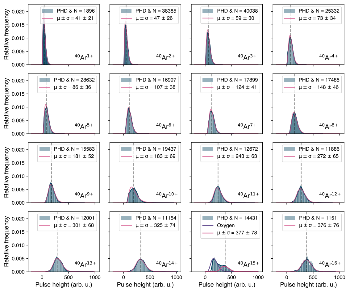
Figure A.4: PHDs of argon at reduced gas pressure. The photon energy is 1100 eV, and the pulse energy on target is 3.2 mJ.
